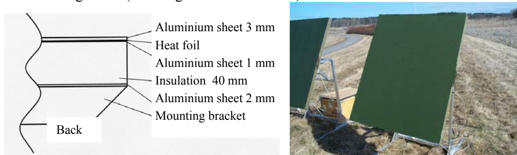
Figure 11 Cross section of the panels and a photo of the two panels on stands (paint panel to the left).
