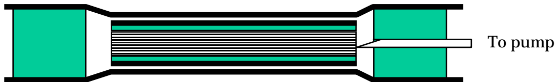
Figure 3. The impregnated weave placed in a heat-shrink tube, sealed with hot glue and evacuated.
