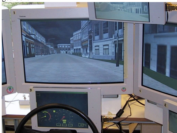
Figure 2: A closer look at the LOCS. Central monitor above LCD-screen with dashboard information (providing speedometer, odometer, rev meter, and indicator lights). Part of the rearview mirror (LCD-screen) is visible.
