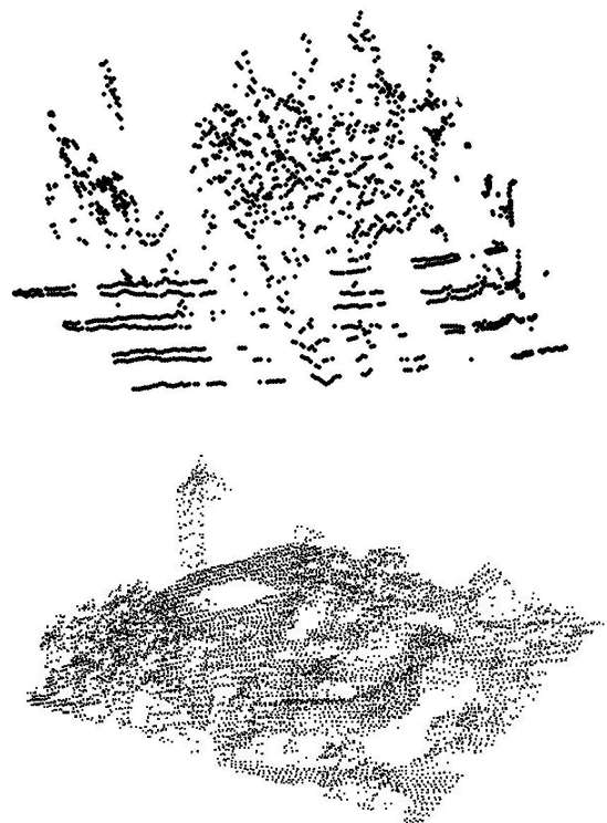
Figure 2. Elevation points from airborne laser scanning. Top: data from a forest area (x and y scales are non-uniform for illustration purposes). Bottom: data from an urban area.
