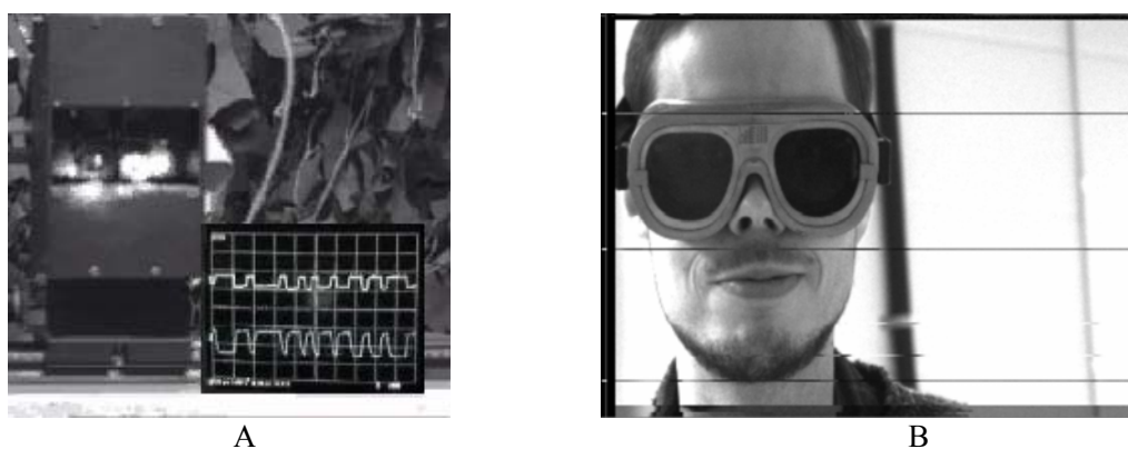
Figure 15 A) Retroreceiver and optical signal detected by the transceiver during tracking. B) Transferred image using the retrocommunication link.
