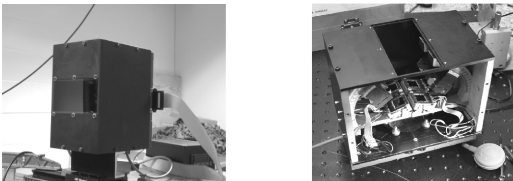
Figure 6 A) Retromodulating receiver assembly. B) Four reflective MQW modulators and retroreflectors constituting the optical assembly. From ref.[10].
