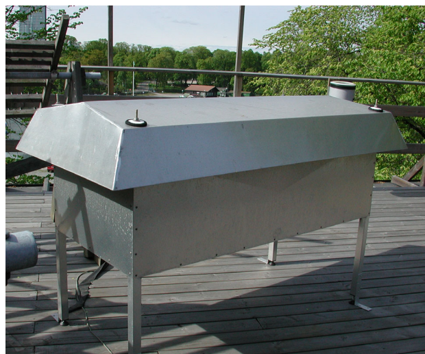
Figure 15. Outdoor exposure of the objects in the second study. The objects were exposed under a weather protective hood.
