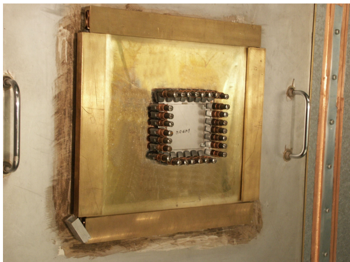
Figure 11. Aperture under test mounted in the reverberation chamber. A brass fixture covers a 290x290 mm opening between two chambers. The test object is mounted, using wave-guide clamps, over an 80x80 mm hole in the common panel brass fixture.
