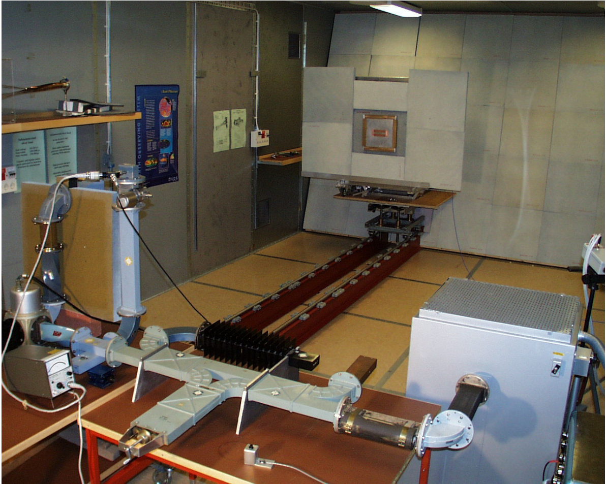
Figure 1. Measurement set-up. 700 kW, 3 GHz, magnetron to the right, transmitting horn antenna to the left. The aperture under test is mounted on a flange on the aluminum box “the kiosk”. In the picture the box is located on the rail at a distance of 4284 mm.
