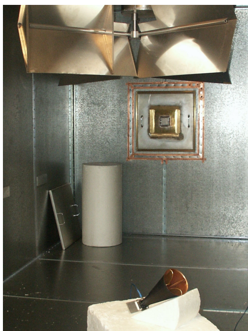
Figure 10. Measurement of aperture transmission cross-section in FOI reverberation chambers. Stirrer in the ceiling, receiving antenna in the front, fixture with test object mounted on a common panel between the two chambers.
