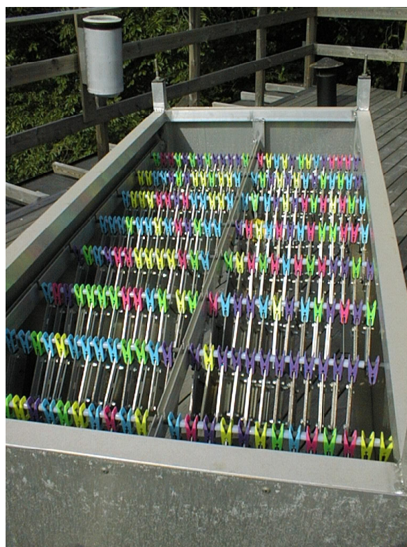
Figure 15. Outdoor exposure of the objects in the second study. The objects were exposed under a weather protective hood.
