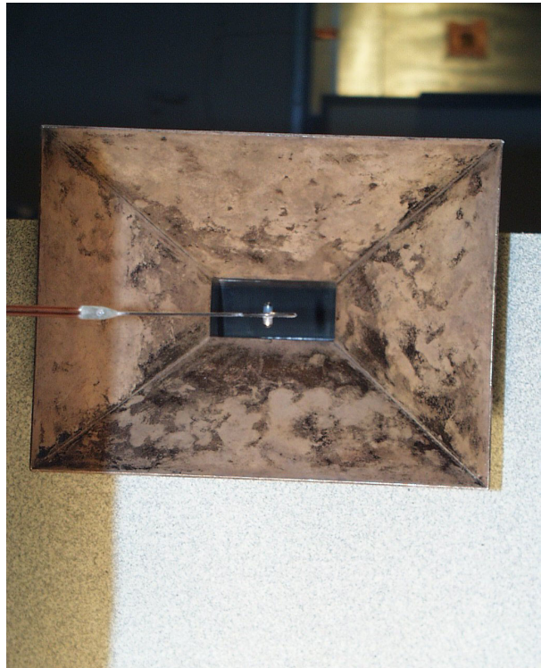
Figure 8. D-dot sensor and transmitting antenna viewed from the aperture under test.
