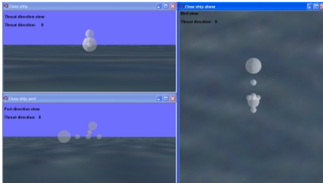
Figure 4.5 Front aspect seen from missile (above to the left). Port view and bird view shows the spheres distribution.
