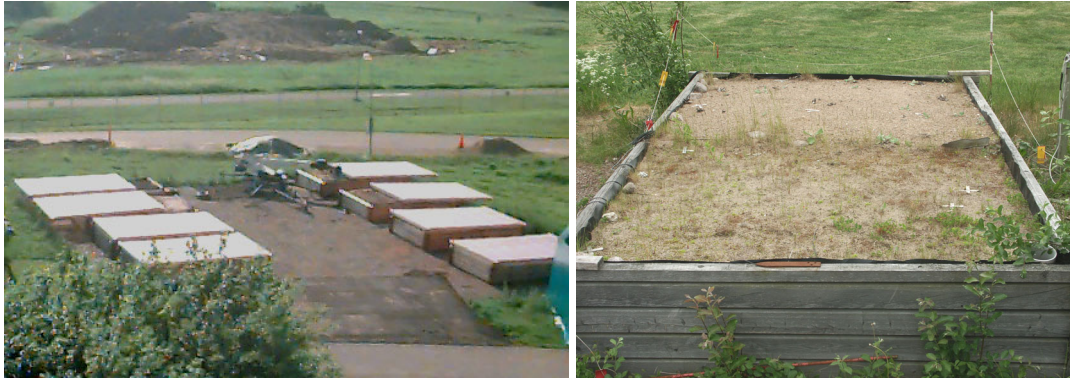
Figure 3.7 To the left: one of eight experimental boxes containing sand in two different grain sizes. Sparse vegetation has been allowed to grow in one part. To the right: a close up.
