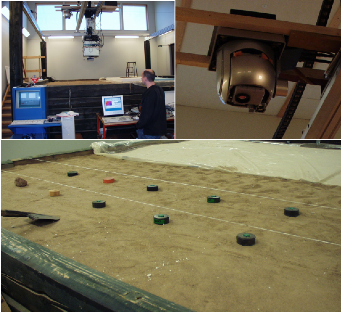
Figure 3.6 Upper left: Large sand box, 4.3x4.3x1.45 m, with high precision XY positioner. Upper right: An example of solution for sensor mounting. Bottom: Objects laid out before burial in sand.
