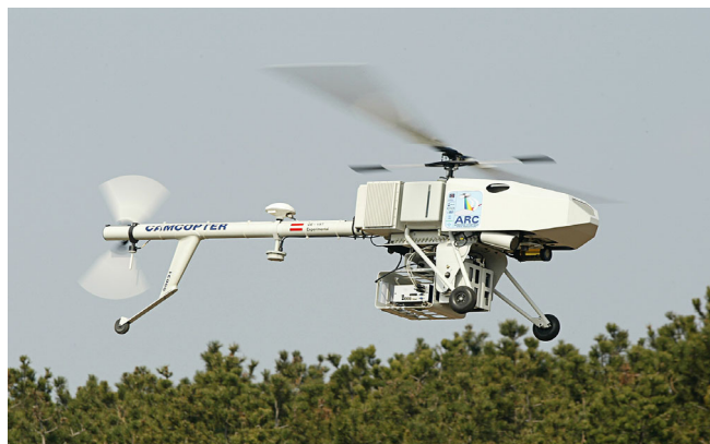
Figure 6.1 UAV used in EU-project ARC as sensor platform for IR and multispectral sensors.
