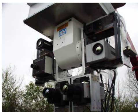
Figure 3.1 Six different optical sensors mounted on the turntable. All useful wavelengths of the optical spectrum are covered.
