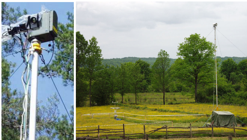
Figure 3.17 Elevated mast with sensors mounted on turntable.
