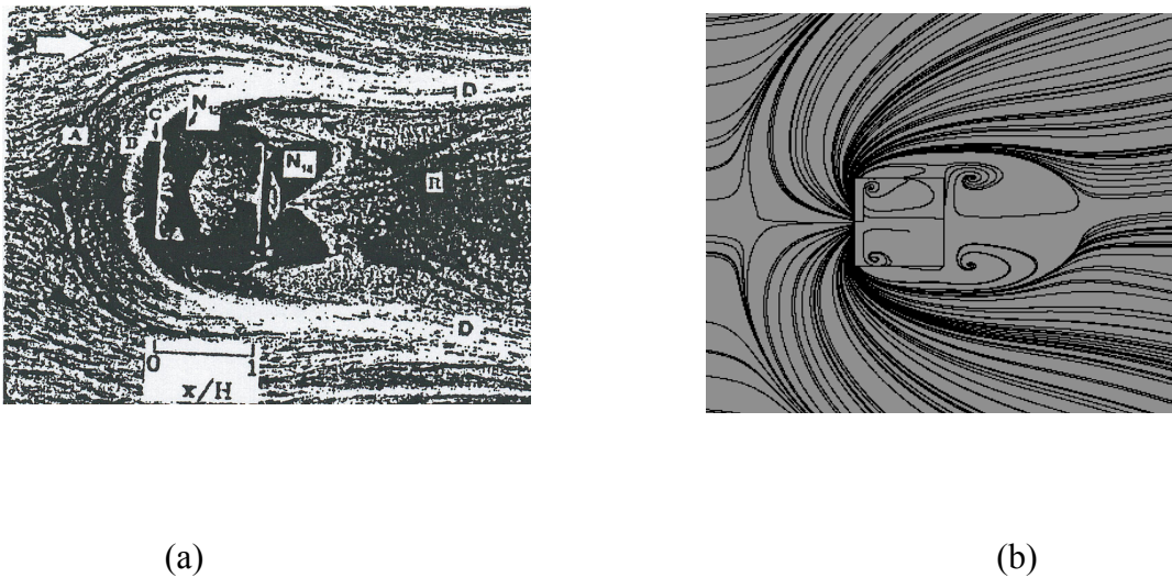
Figure 16. Surface streamlines in (a) experiment (Martinuzzi and Tropea, 1993) and (b) in OEEVM with wall model, fine grid. We see a clear discrepancy in the surface streamline patterns of the simulation and the experiment. The influence region of the cube in the surface streamline pattern is much larger in the simulation compared to the experiment.
