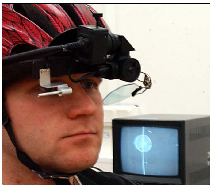
Figure 1. The Mooij Holding GazeTracker II, an Eye-Point-of-Gaze equipment.
