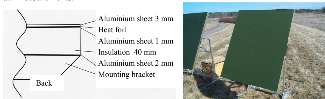
Figure 7 Cross section of the panels and a photo of the two panels on stands (paint panel to the left).
