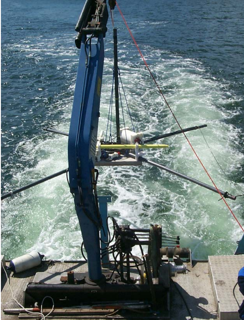
Figure 2. Three-axis short baseline electrode system. Electrodes are at the ends of the grey plastic pipes. The long, thin, yellow rod is one of the magnetic coils. Compass and tiltmeters are in the small pod and amplifiers in the big one.
