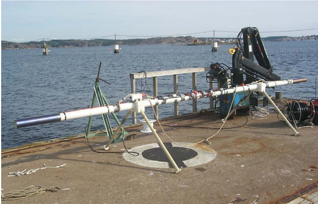
Figure 3. Stationary electric source with titanium electrodes at each end. The small pod above two of the legs contains compass and tiltmeters.
