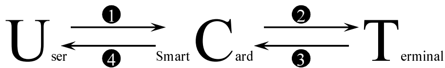
Figure 7: The traditionally identified entities involved in a smart card-based authentication process, that is, the user, smart card, and terminal. The numbered edges represent the authentication steps used to establish a chain of trust between these entities.
