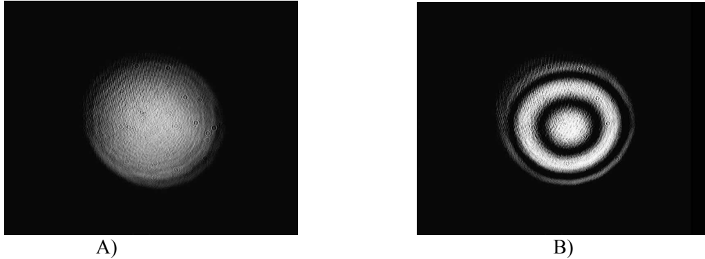
Figure 10 A) Null interferogram corresponding to the DM mirror with no voltage applied to the actuators. B) Null interferogram with 140V applied to the 20 central actuators of the DM.
