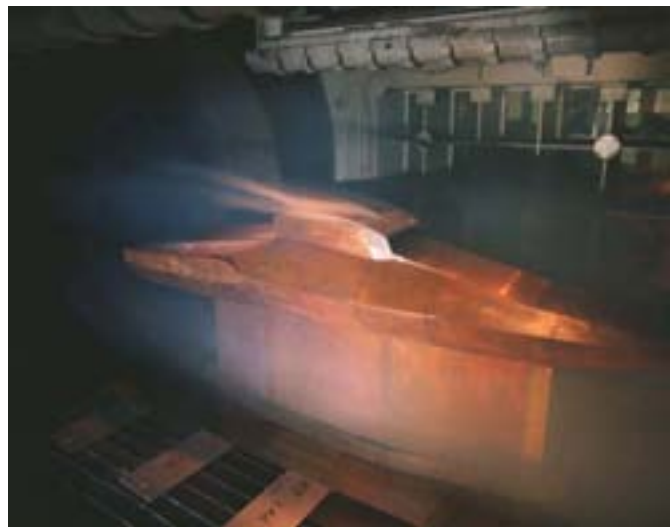
Figure 54. Wind tunnel model of X 43 showing inlet, combustion chamber and exit.
