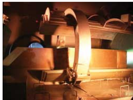
Figure 4. Test firings of the scramjet engine in Japan at Ma 8 flight conditions. Photo taken from //www.aiaa.org/aerospace/Article.cfm
