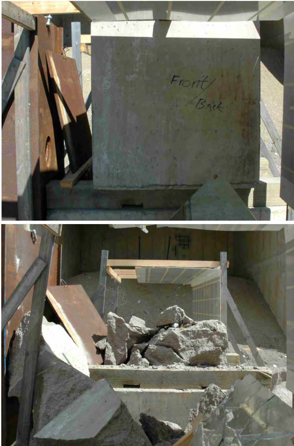
Figure 3.40. Normal strength concrete target without confinement and reinforcement before and after test number 2004-21.
