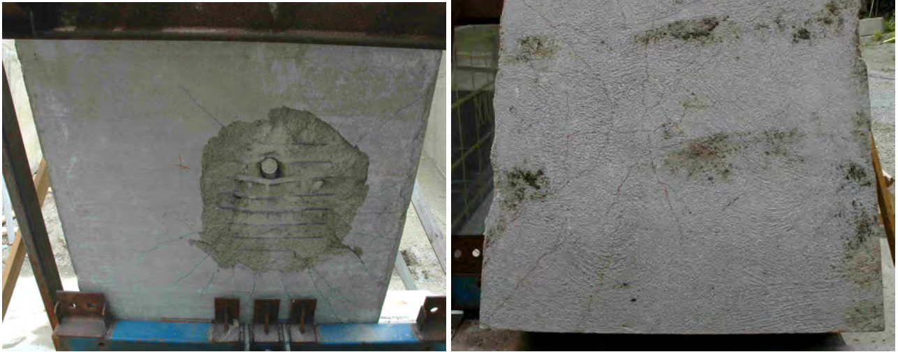
Figure 3.54. Reinforced normal strength concrete target after test number 2004-23-2. This is the first test in target 2004-23.
