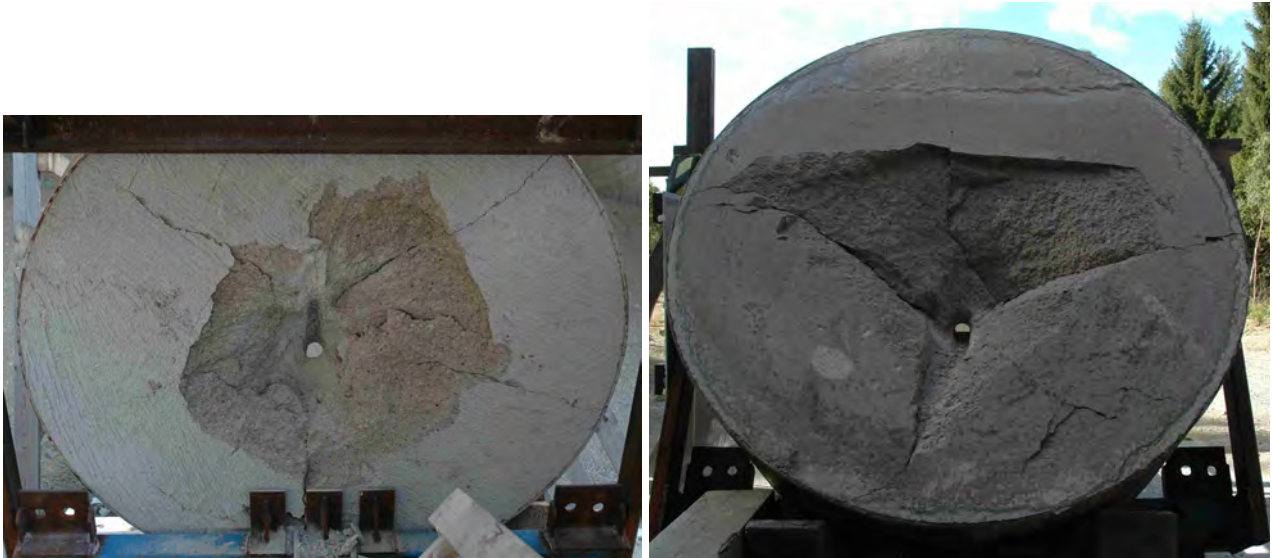
Figure 3.45. Normal strength concrete targets after test number 2004-25.
