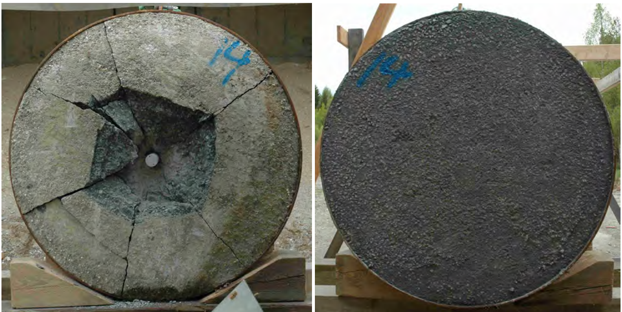
Figure 3.30. High performance concrete target after test number 2004-14, front and back views.
