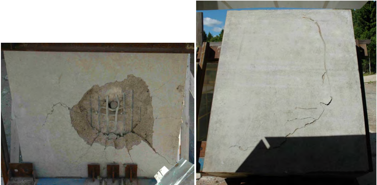
Figure 3.58. Reinforced normal strength concrete target after test number 2004-24-1. This is the first test in target 2004-24.
