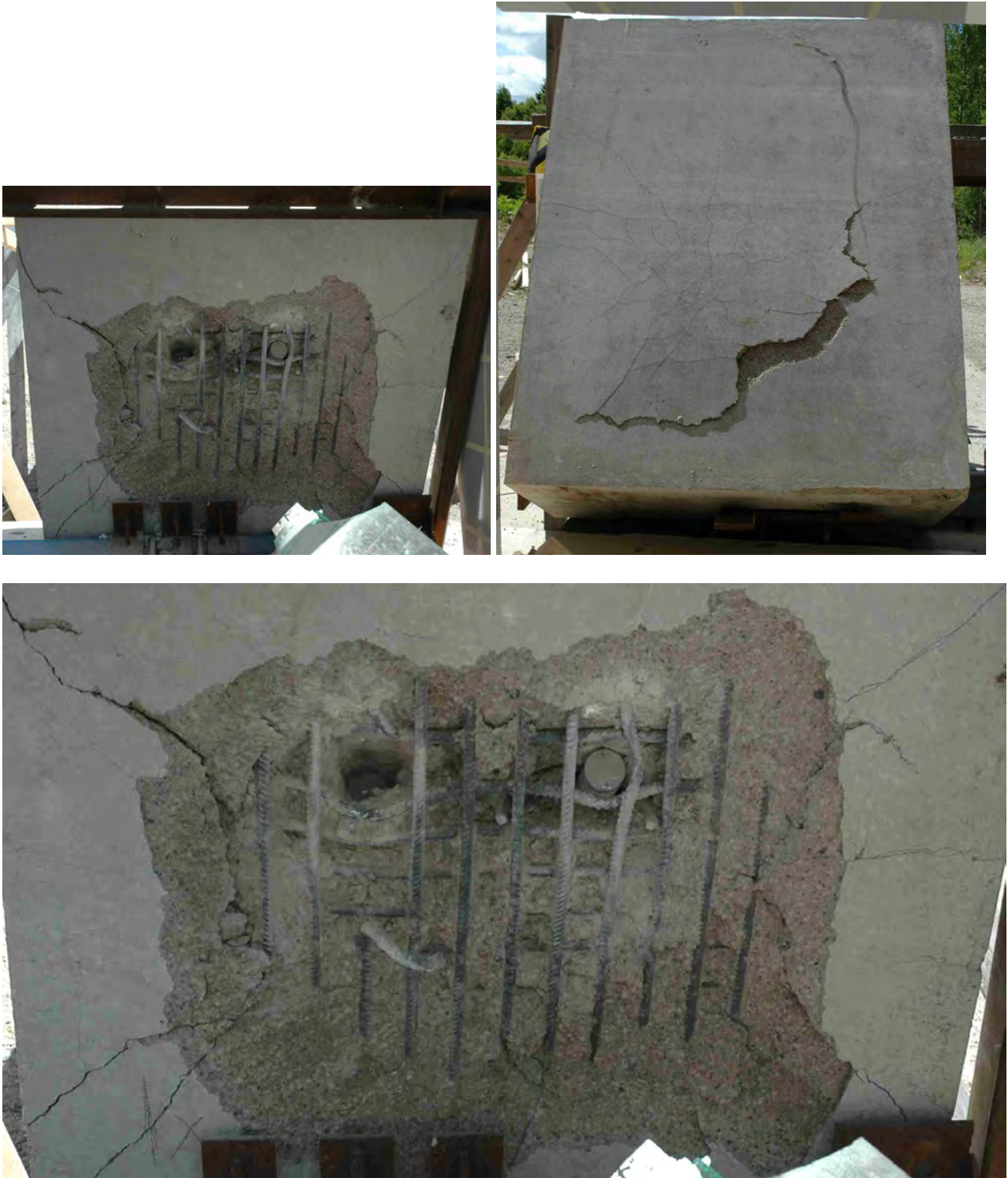
Figure 3.59. Reinforced normal strength concrete target after test number 2004-24-2. This is the second test in target 2004-24.
