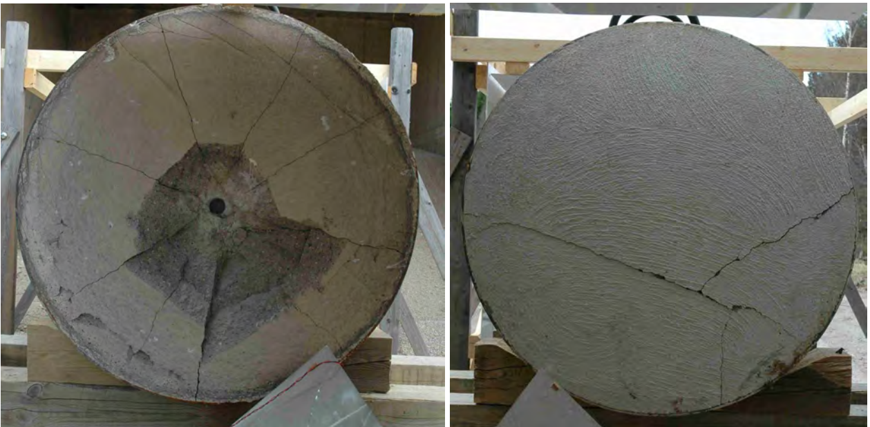
Figure 3.21. Normal strength concrete target after test number 2004-3, front and back views.
