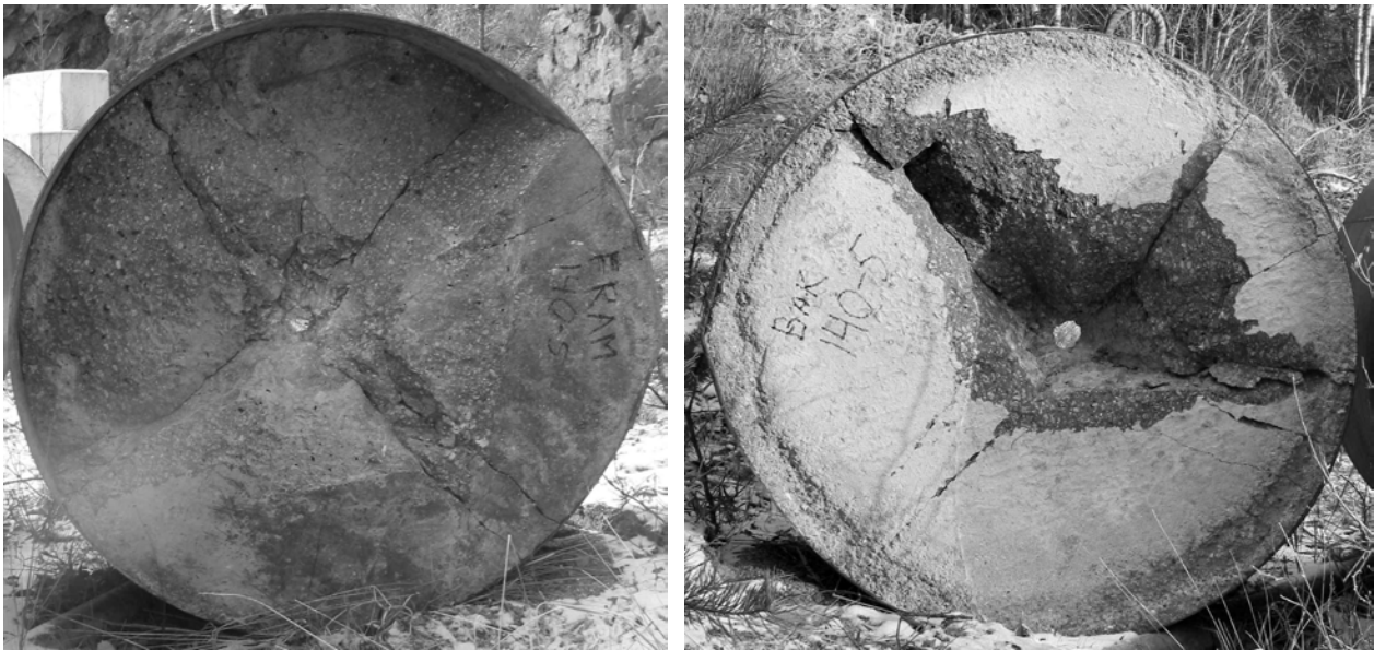
Figure 3.12. Target from test number 2002-11 with HPC K140 concrete, front face to the left and back face to the right.
