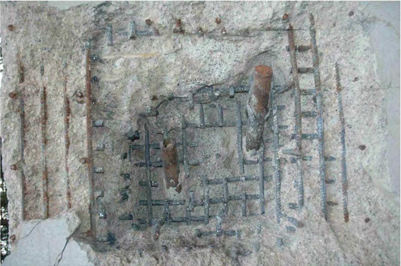
Figure 3.60. Reinforced normal strength concrete target 2004-24 shown during removal of the projectiles. The projectile from test no. 2004-24-1 is shown to the right.
