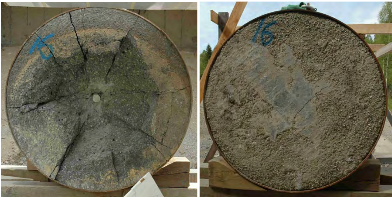
Figure 3.32. High performance concrete target after test number 2004-16, front and back views.
