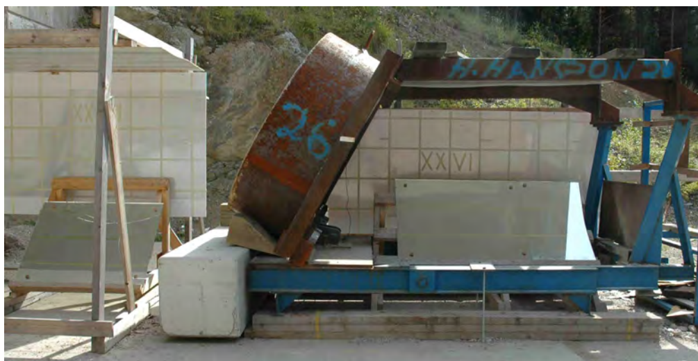
Figure 2.7. Target placement for the tests with approximately 90° and 60° impact angles. The positions of the short circuit screens for velocity measurement are also shown in the upper figure, with a third short circuit screen mounted on the surface of the target.
