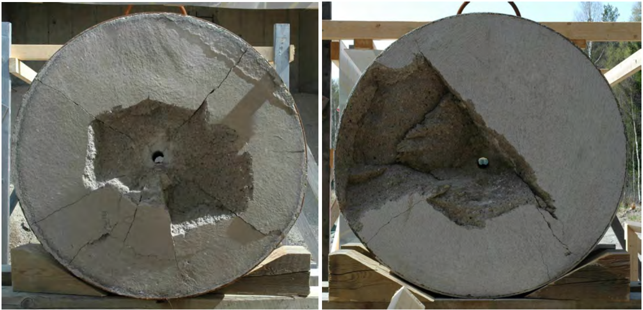
Figure 3.24. Normal strength concrete target after test number 2004-6, front and back views.
