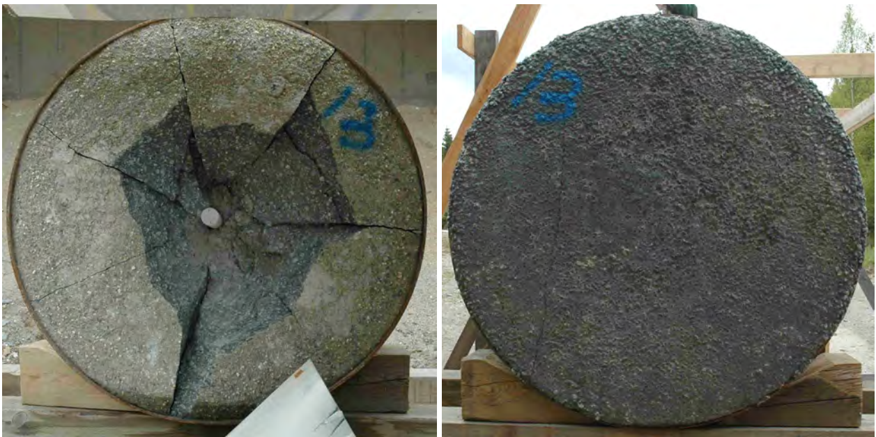
Figure 3.29. High performance concrete target after test number 2004-13, front and back views.
