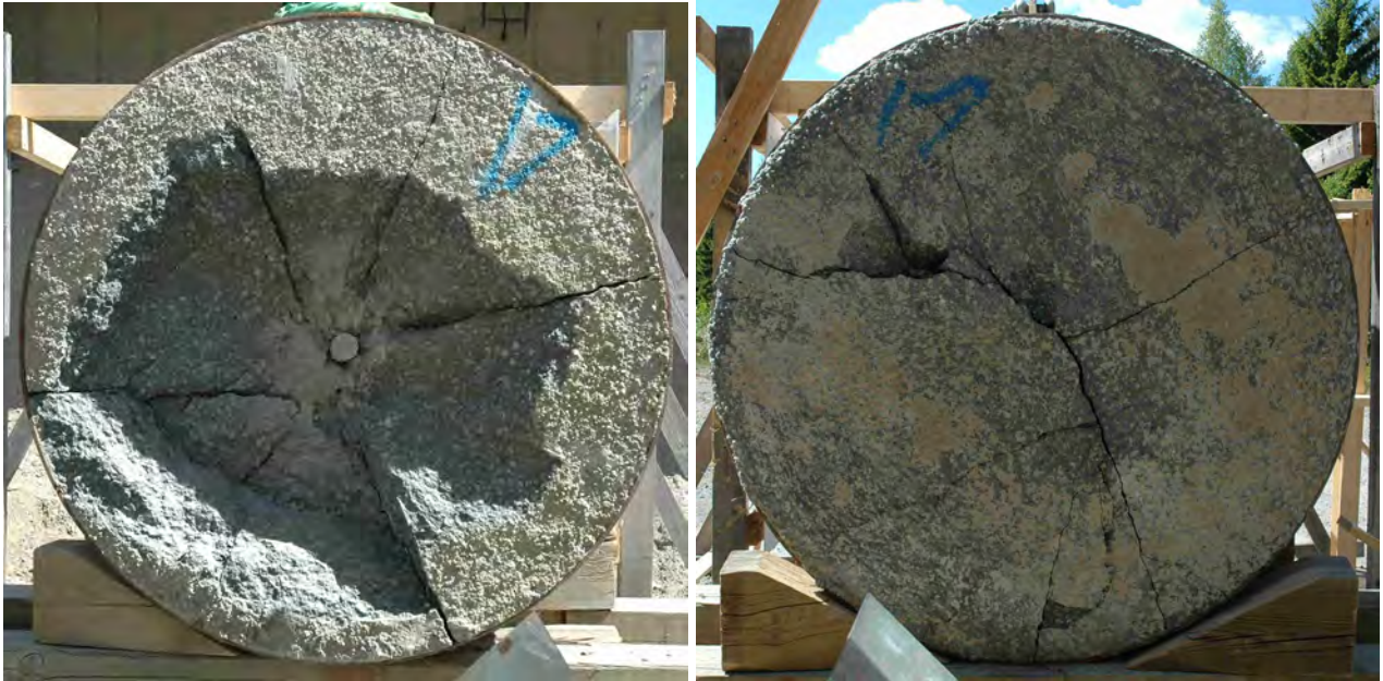
Figure 3.34. High performance concrete target after test number 2004-17, front and back views.
