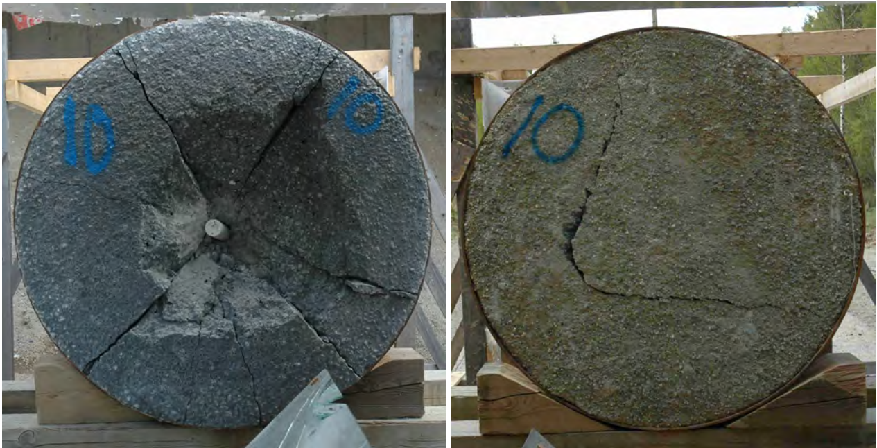
Figure 3.27. High performance concrete target after test number 2004-10, front and back views.
