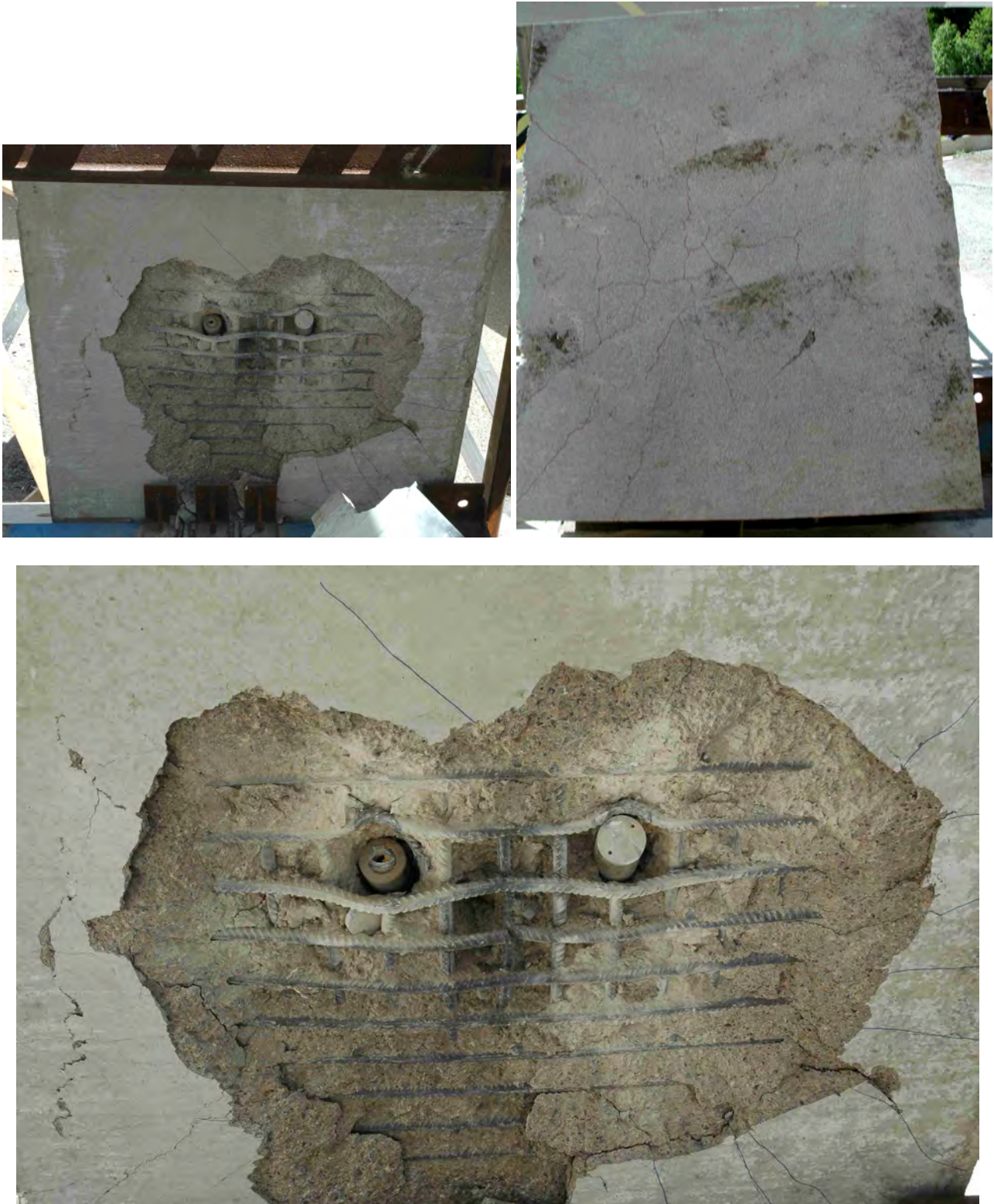
Figure 3.55. Reinforced normal strength concrete target after test number 2004-23-1. This is the second test in target 2004-23.
