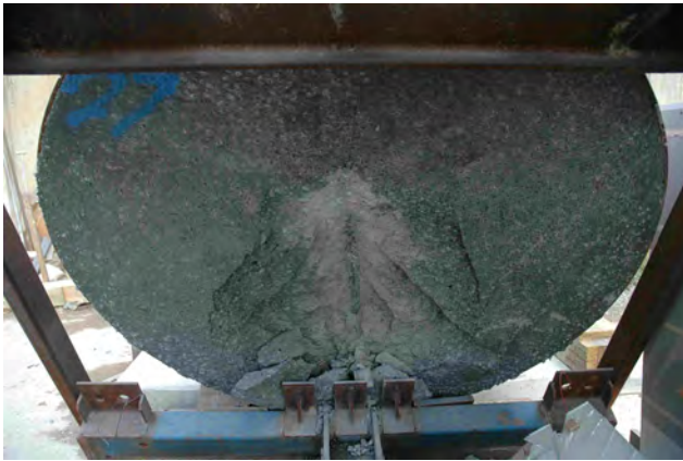
Figure 3.50. High performance concrete target after test number 2004-27.
