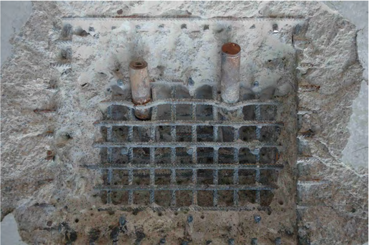
Figure 3.56. Reinforced normal strength concrete target 2004-23 shown during removal of the projectiles. The projectile from test no. 2004-23-2 is shown to the right. Projectile 2004-23-1 shown to the left is broken into two pieces, this was the second test in the target.
