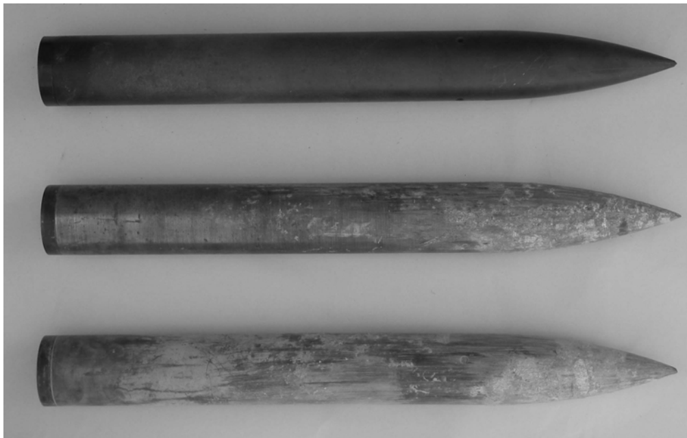
Figure 3.6. Projectiles after tests compared with an unfired projectile, from top unfired projectile, test projectiles 2002-1 and 2002-2.
