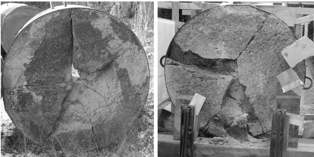
Figure 3.13. Target from test number 2002-12 with HPC K140 concrete, front face to the left and back face to the right.
