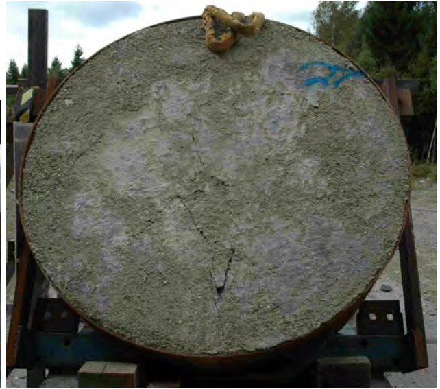
Figure 3.50. High performance concrete target after test number 2004-27.
