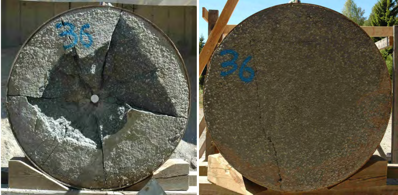
Figure 3.33. High performance concrete target after test number 2004-36, front and back views.
