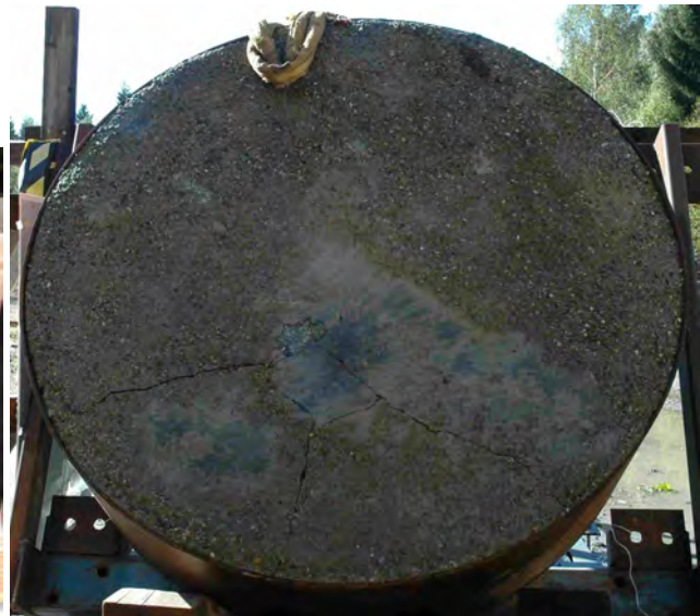
Figure 3.51. High performance concrete target after test number 2004-28.
