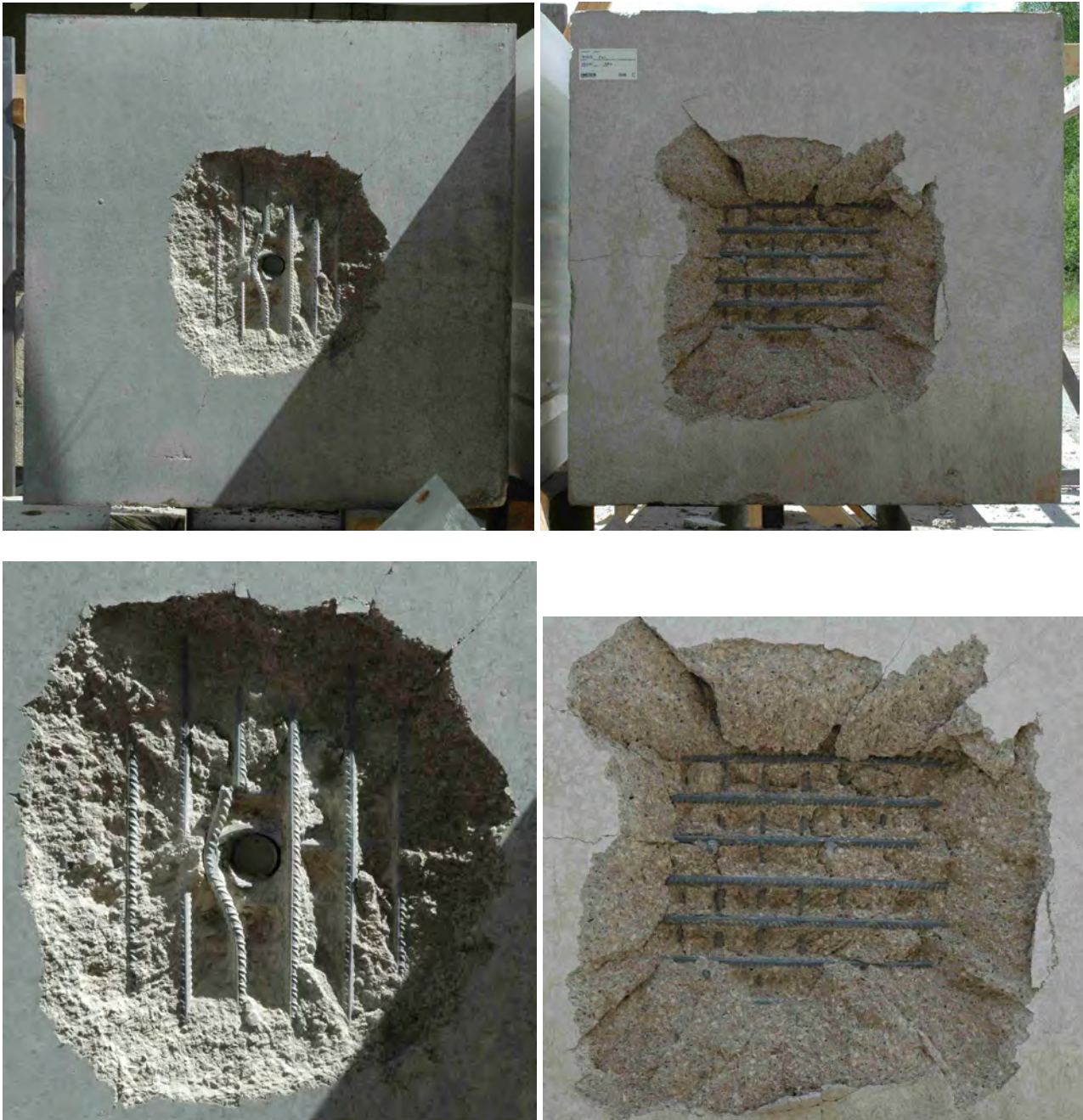
Figure 3.37. Reinforced normal strength concrete target after test number 2004-20, incl. details of craters. Front views to the left, and back face shown to the right.
