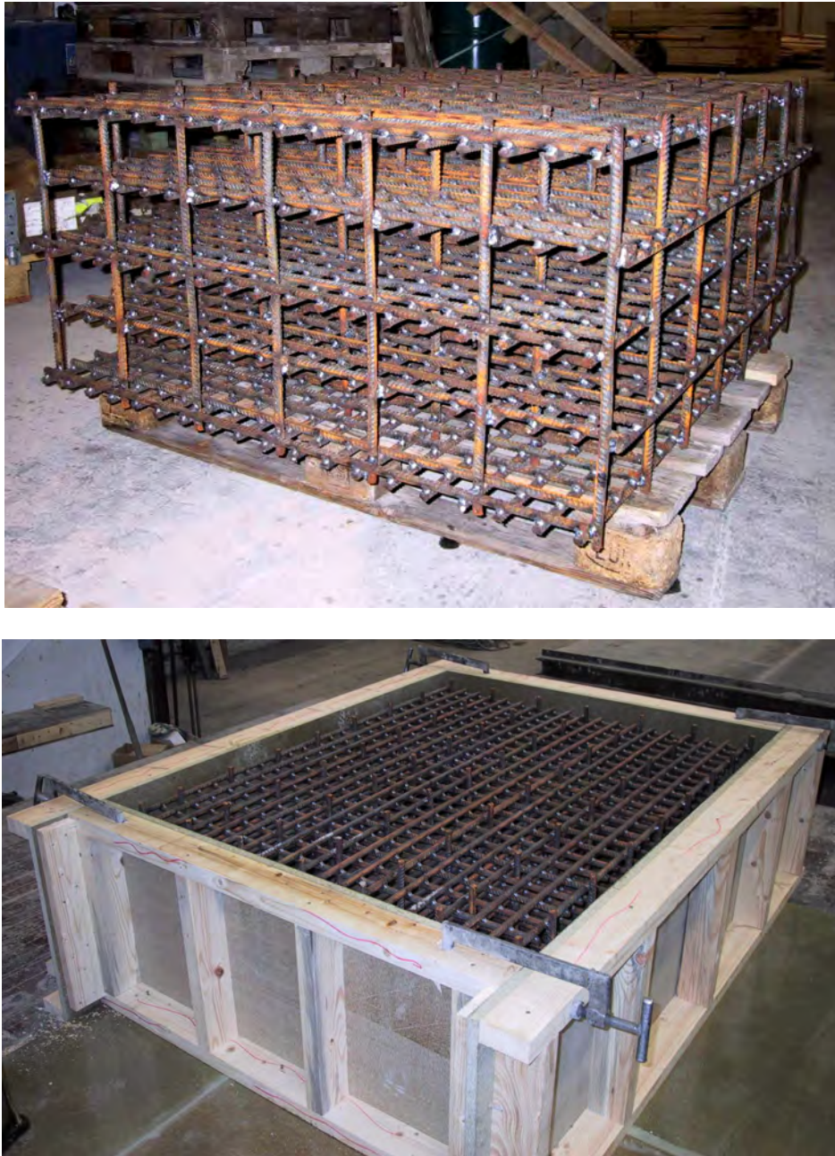
Figure 2.4. Example of welded reinforcement cages for targets used in tests performed in 2004.
