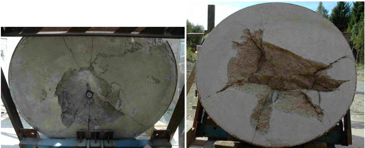
Figure 3.46. Normal strength concrete targets after test number 2004-26.
