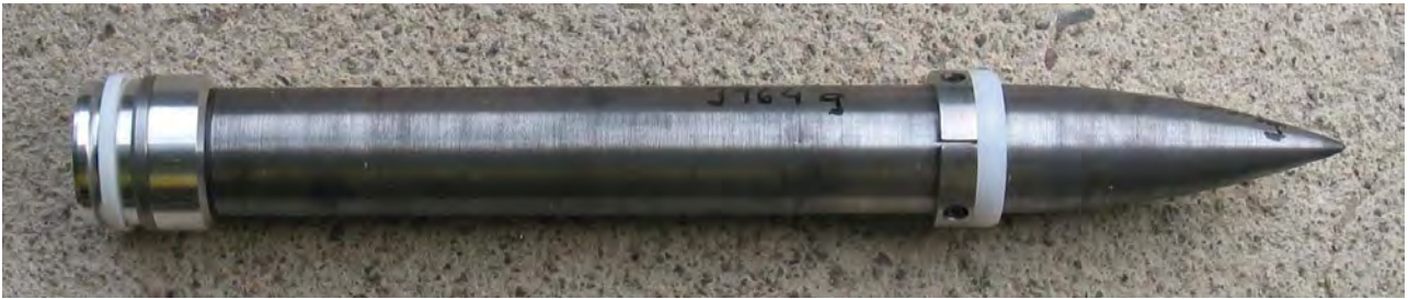
Figure 2.1. The used types of projectiles for the test, (a) the three different nose shapes of the projectiles used in 2004, and (b) the 50 mm diameter projectile shown with guidance ring and aluminium pusher plate. The masses of the guidance ring and pusher plate are approximate 130 and 350 g, respectively.
