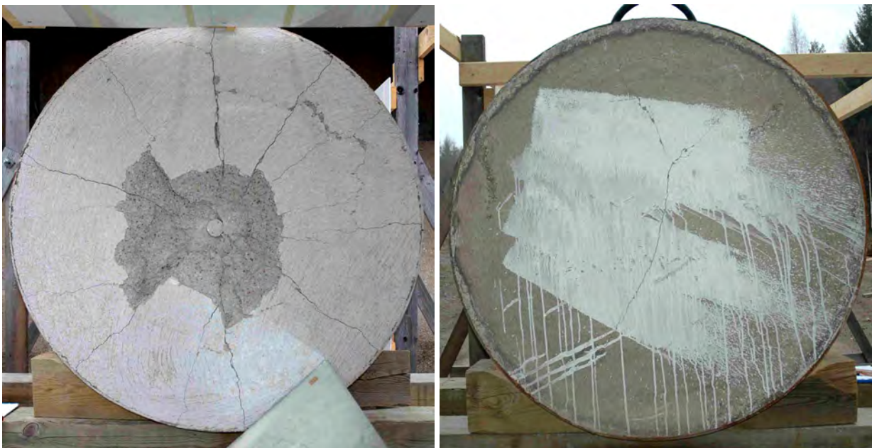
Figure 3.19. Normal strength concrete target after test number 2004-1, front and back views.
