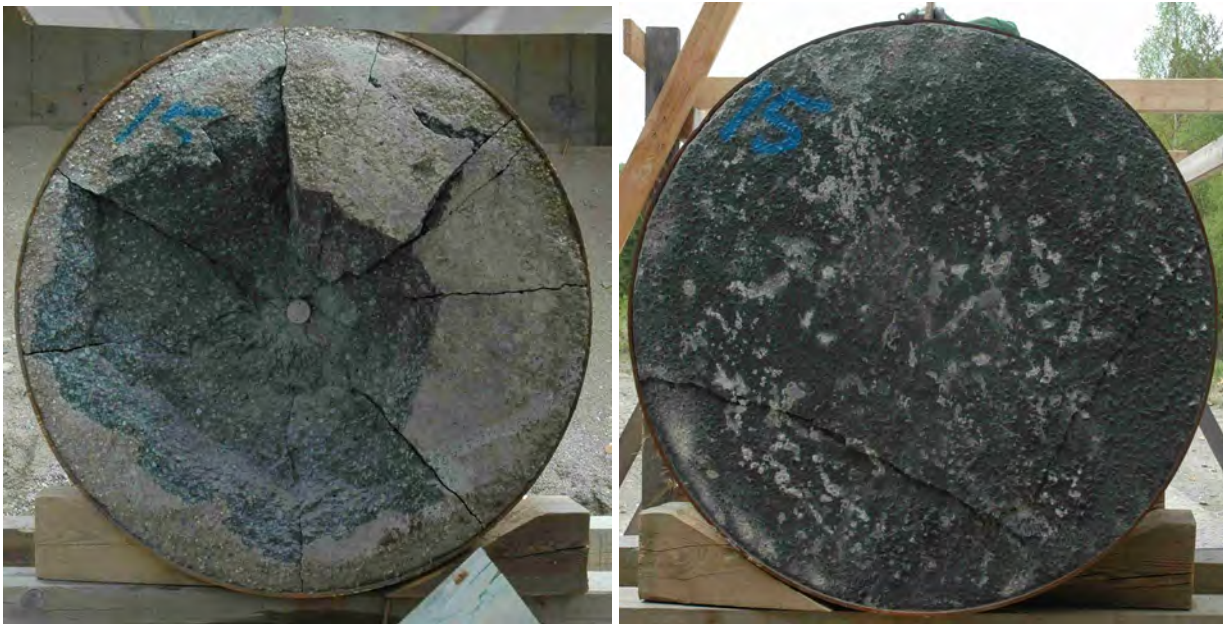
Figure 3.31. High performance concrete target after test number 2004-15, front and back views.
