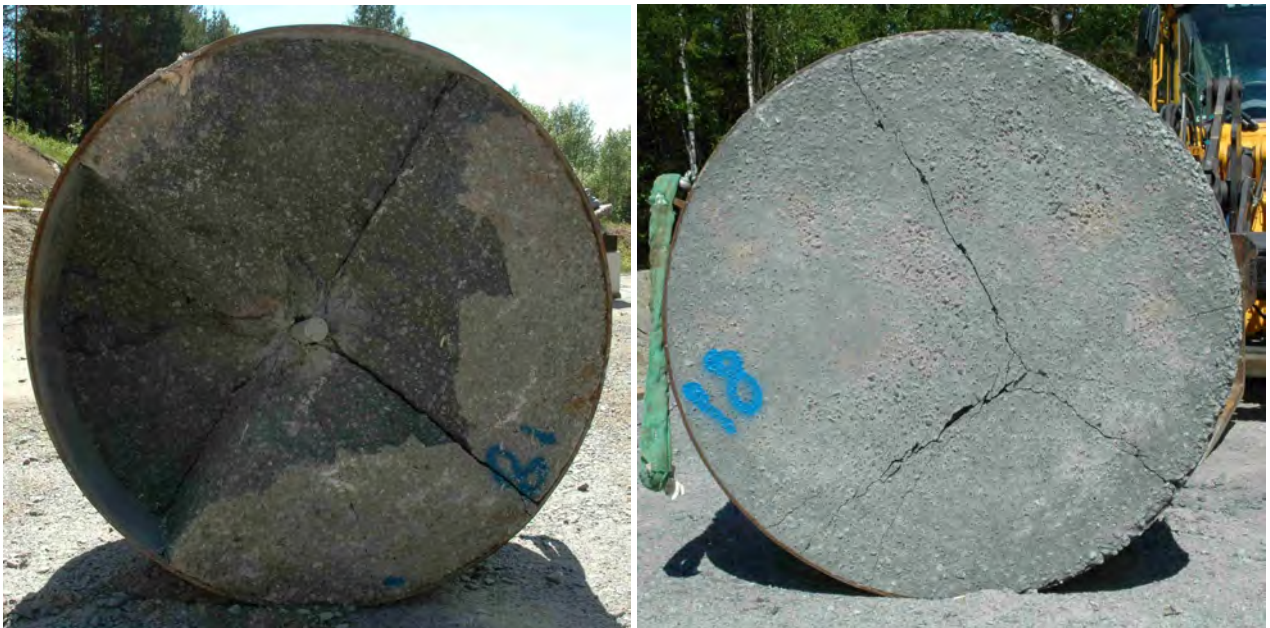
Figure 3.35. High performance concrete target after test number 2004-18, front and back views.
