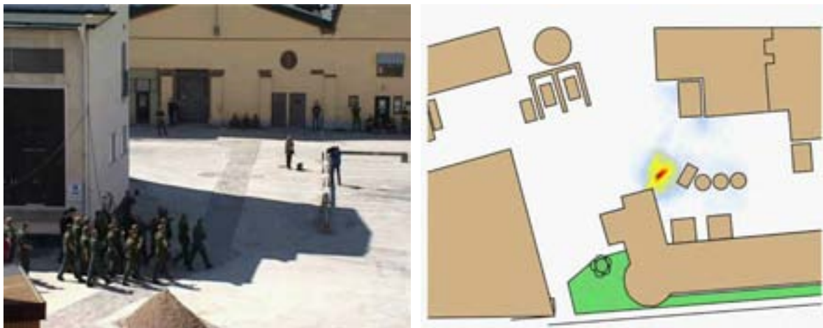
Figure 3.2: Localization of people using acoustic sensors.
