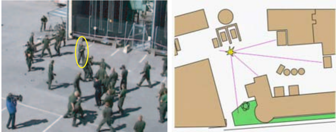
Figure 3.1: Localization of gunfire using acoustic sensors.
