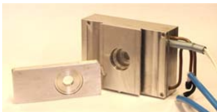
Fig.4 The temperature chamber that was used in the FTIR. The sample was placed in the sample holder to the left in this picture.
