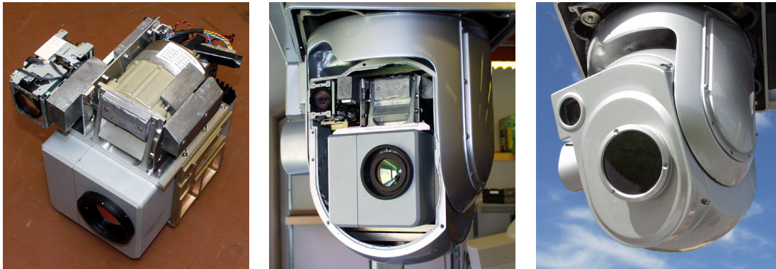
Figure 6.1. The gimbal system. Left: Inner gimbal consists of an IR camera and a color CCD. Middle: The gimbal with demounted front. Right: Gimbal with mounted front.
