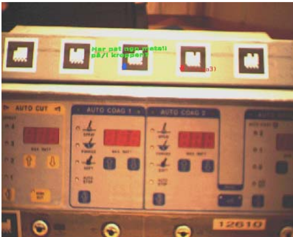
Figure 4.2 Image of the mock-up of the Diathermy Apparatus with markers. The blue hand below the question indicates that this question has to be answered before moving on. The marker next to it will only display a red message indicating that the previous step has to be completed before the next instruction will appear.
