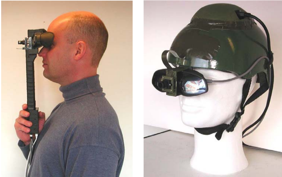
Figure 3.2 Video-See-Through MR-units. To the left a hand-held unit developed in the present phase and to the right the head-wearable unit developed in the previous phase.
