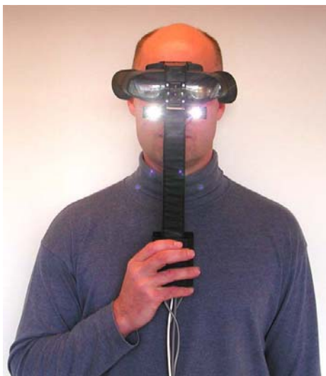
Figure 3.3 A hand-held MR-unit with lighting possibilities.
