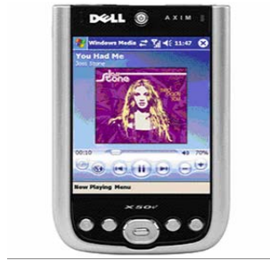
Figure 3.20 The handheld computer Axim X50V with VGA output, wireless LAN and 3D graphics hardware support.
