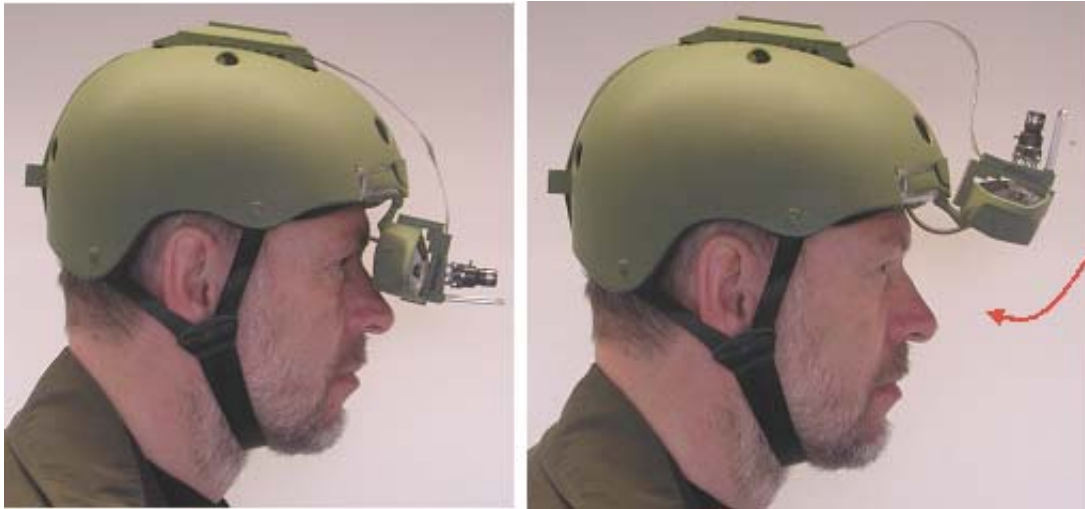
Figure 3.5 Different modes, down or turned up, of using the video-see-through unit.
