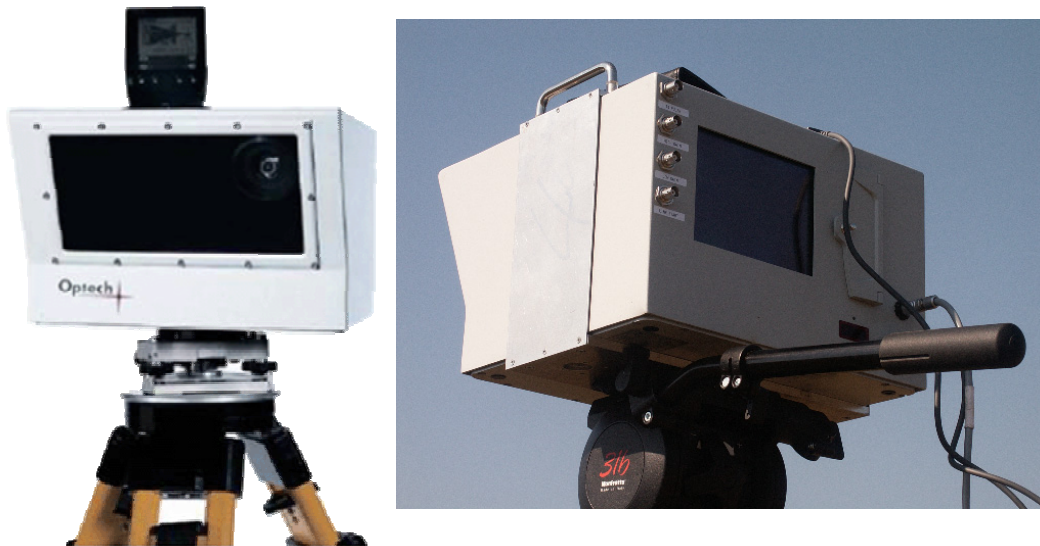
Figure 8-18. The laser scanner ILRIS-3D, front view to the left. The measurement head is mounted on a tripod. On top is the PalmPilot, which is connected to the measurement head with a cable. The photo to the right shows the display window on the back of the measurement head.
