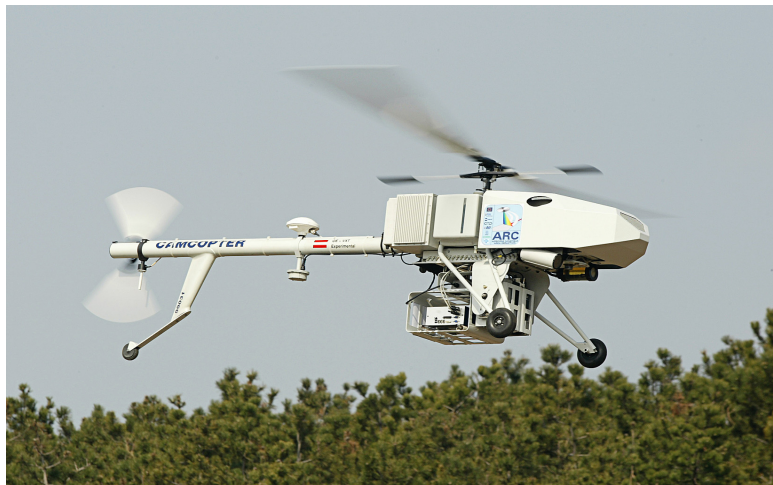
Figure 7-6 ARC UAV with IR and multispectral sensors.
