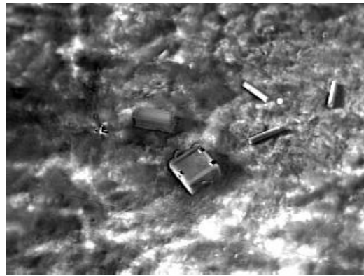
Figure 5-7 Time constant from a sequence of IR frames. In (a), the first frame of a sequence is shown, and in (b), the time constant image is shown. In (a) bright parts correspond to a high apparent temperature and dark parts to low apparent temperature. In (b) bright parts correspond to high time constant and dark parts to low time constant.
