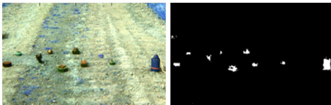
Figure 4-55. Left: RGB-rendering of hyperspectral image. Right: Information based target detection based on hyperspectral data.
