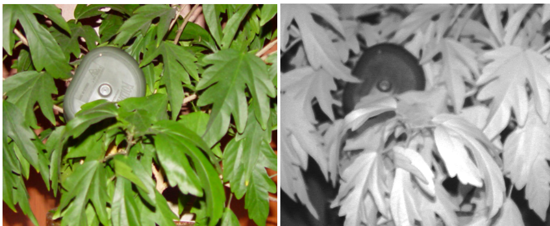
Figure 4-53. Left: Green plastics in vegetation as viewed in reflection with a RGB sensor. Right: Green plastics in vegetation as viewed in reflection with a NIR sensor.
