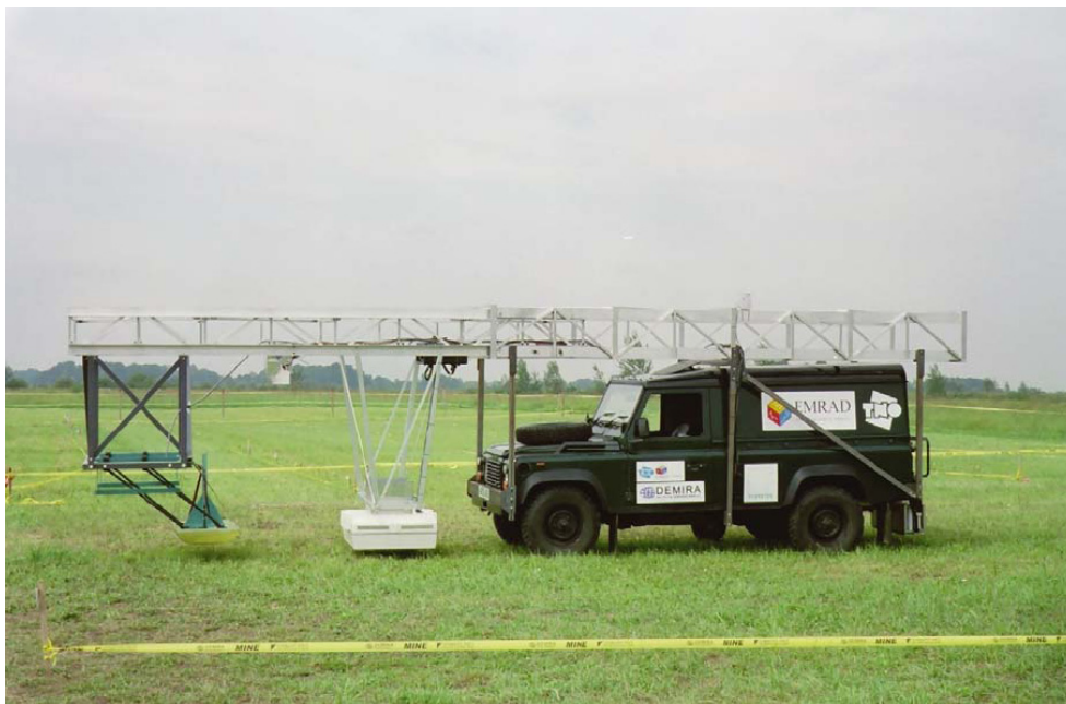
Figure 7-8. The LOTUS Vehicle. The metal detector is at the front, as far away from the vehicle and other metal as possible. The infra-red camera then follows within the framework and the GPR array is then immediately in front of the vehicle.
