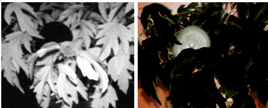
Figure 4-54. Left: Green plastics in vegetation as viewed in fluorescence with a NIR sensor. Right: Green plastics in vegetation as viewed in reflection with a RGB sensor and fluorescence suppression mask.
