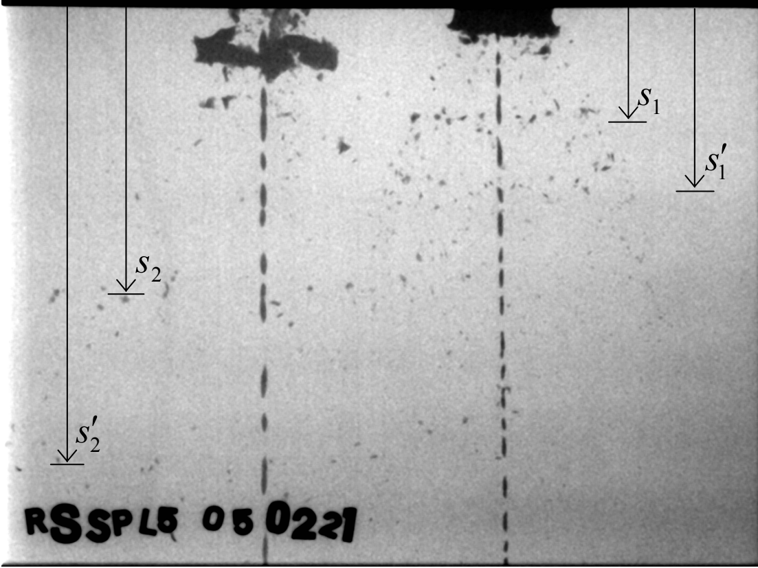
Figure 2. Original radiograph of SC jet and target fragments with 70 \mu\text{s} delay between the first photo (to the right) and the second (to the left). Same scale as in Figure 3 below.
