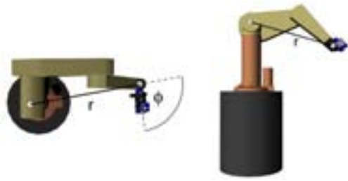
Fig. 1: Top and side view of the platform with parameterization used for constrained path planning
