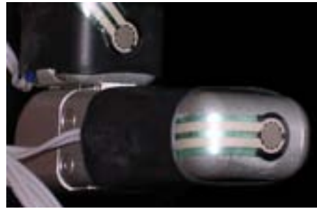
Fig. 2. Force sensing resistors mounted to a finger link and to the fingertip on the finger of a Barrett hand.
