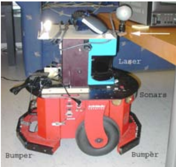
Fig. 1. “Goofy” in collision (see top right corner) with a table. This is not observable by the laser scanner (blue), sonars or the bumper switches since they are vertically displaced compared to the table.
