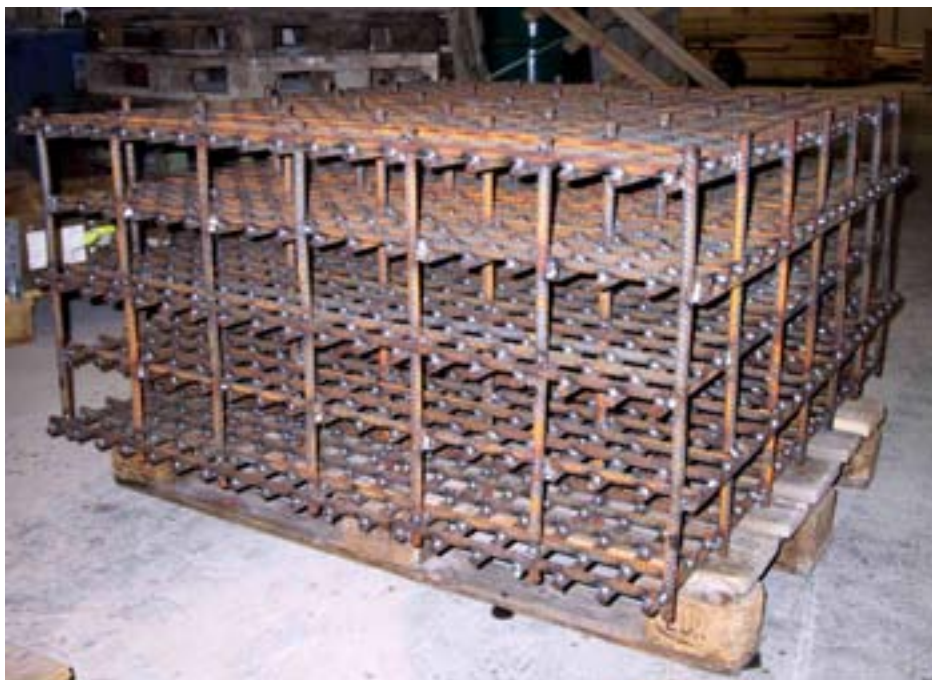
Figure 3.47. Example of a welded reinforcement cage for a 1.2 \times 1.2 \times 0.6 m target used in tests performed during 2004.
