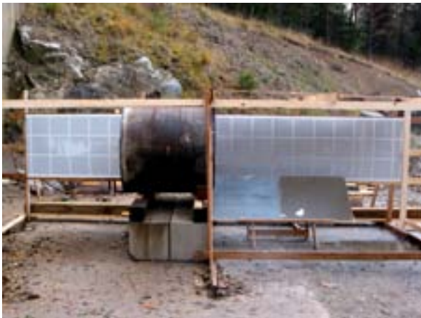
Figure A3.4. Target placement for the test series conducted in 2002. The positions of the short circuit screens for velocity measurement are also shown.
