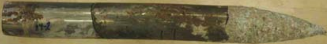
Figure A3.23. Recovered projectiles from target number 3004-24. Both of the projectiles were broken into two pieces, with the projectile from test 2004-24-2 fractured approximately 10 cm from the nose and the projectile from test 2004-24-2 fractured approximately 13 cm from the back face.
