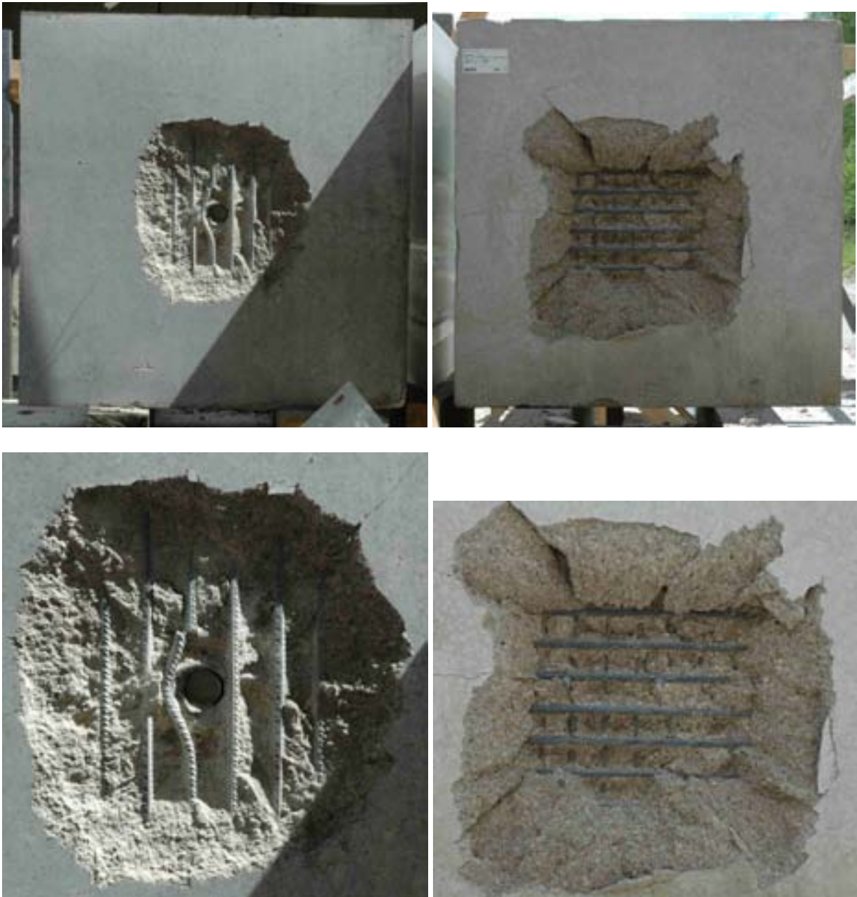
Figure A3.13. Reinforced normal strength concrete target after test number 2004-20, incl. details of craters. Front views to the left, and back face shown to the right.
