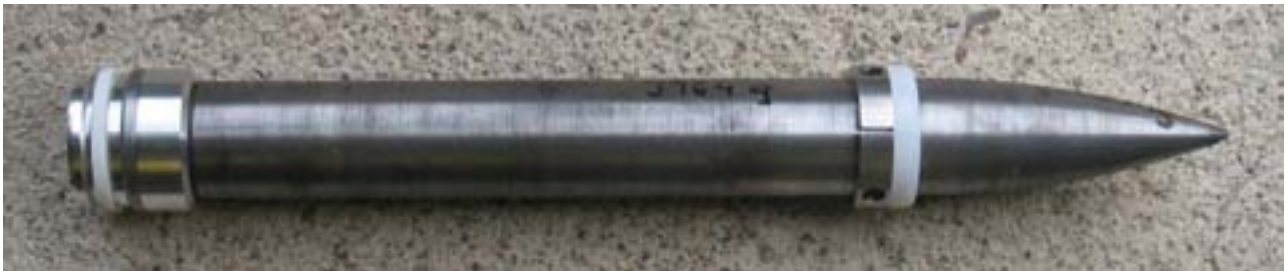
Figure A3.1. The 50 mm diameter model scale projectile shown with guidance ring and aluminium pusher plate. The masses of the guidance ring and pusher plate are approximate 130 g and 350 g, respectively.
