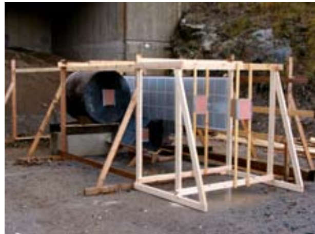
Figure A3.4. Target placement for the test series conducted in 2002. The positions of the short circuit screens for velocity measurement are also shown.
