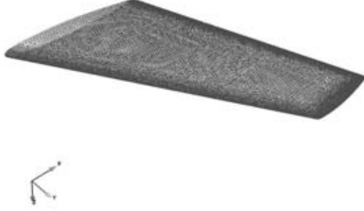
Figure 3.1: Euler mesh on the ONERA M6 wing.
