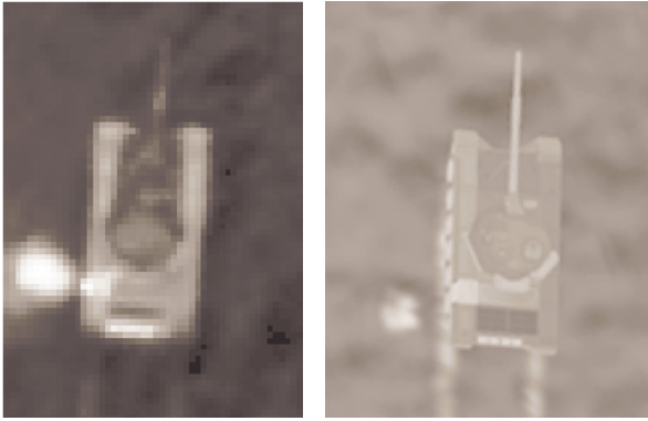
Figure 13: Models for exhaust plume and vehicle tracks are included in the IR-model library. Left: IR image of a T-72. Right: IR model of the T-72 with activated models for exhaust plume and vehicle trails.
