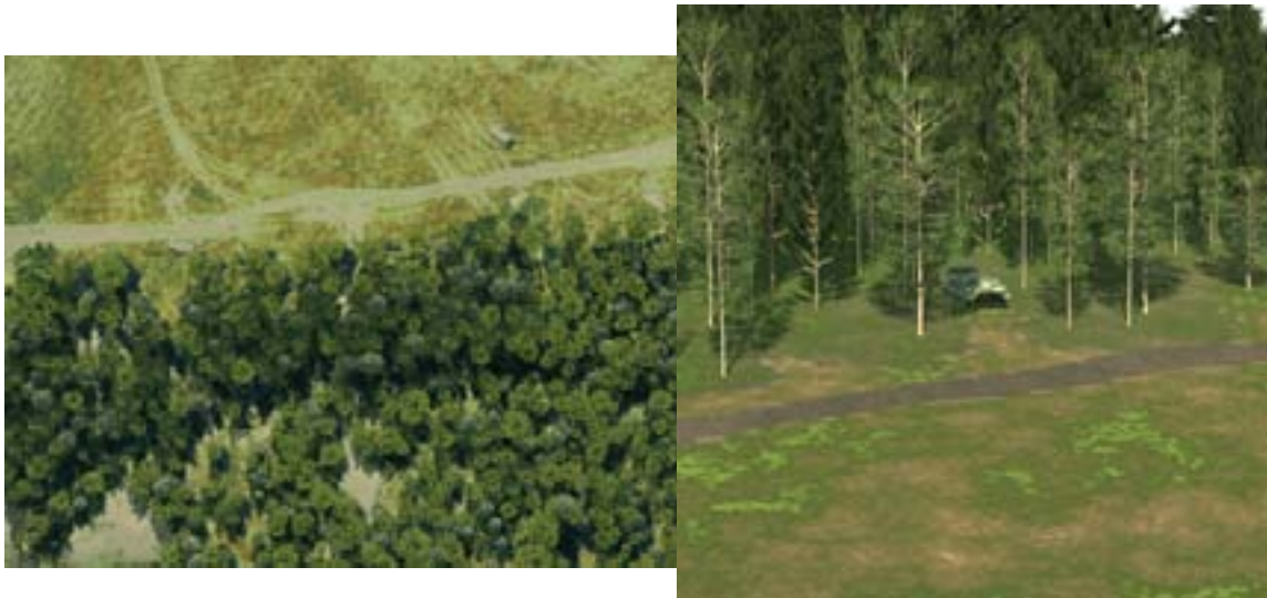
Figure 12. Terrains created using RGB-images (left), and using procedural textures (right).
