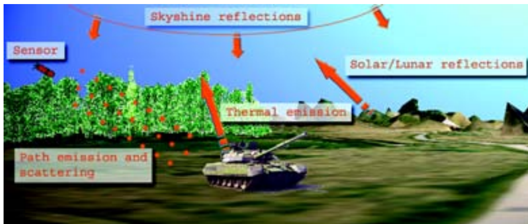
Figure 5 Schematic illustration of some important components included in radiometric calculations.
