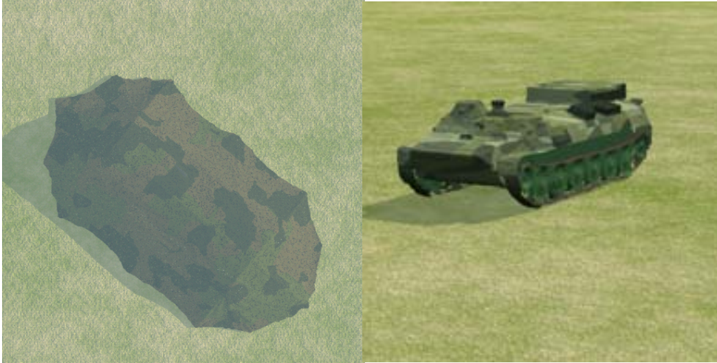
Figure 24. Synthetic simulated camouflage net with Pbv 401 underneath (left) seen from 1500 m, and a Pbv 401 with an averaging camouflage pattern (right).
