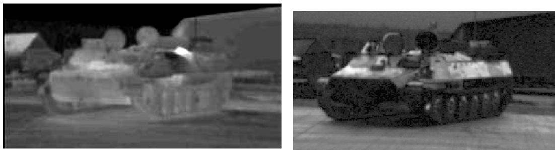
Figure 18. The vehicle measured without polarizer (left). DoLP of the vehicle (right).
