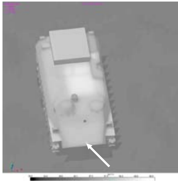
Figure 31. Pbv 401 with element 7691 highlighted in white. Scale is in physical temperature.
