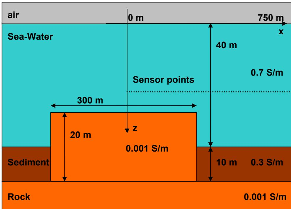
Figure 2. The geometry of the shallow water marine environment model.
