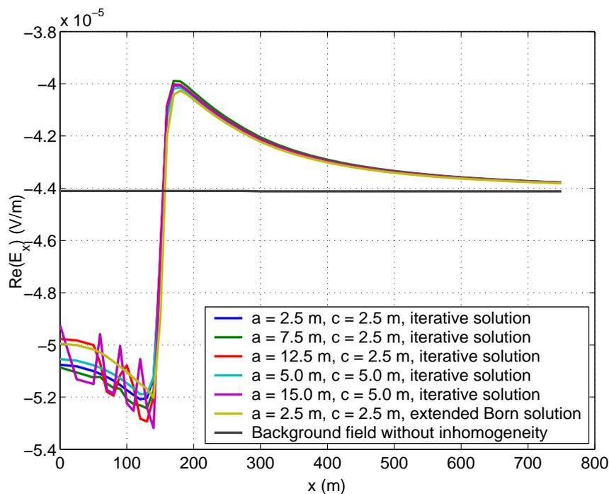
Figure 3. The real part of the horizontal electric field component along the sensor line.
