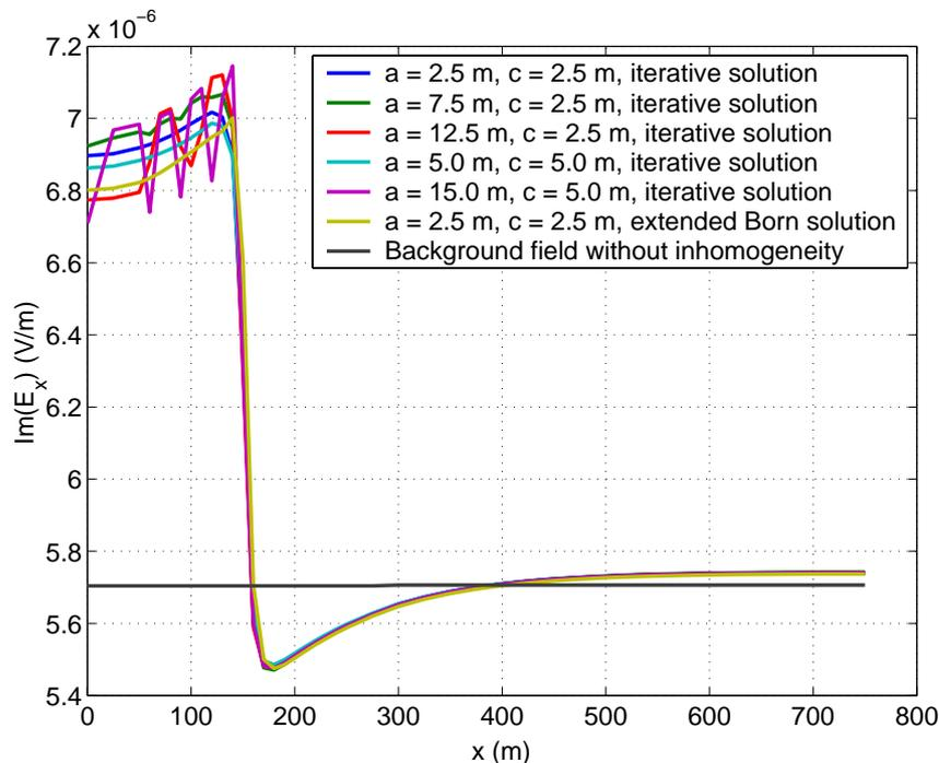
Figure 4. The imaginary part of the horizontal electric field component along the sensor line.
