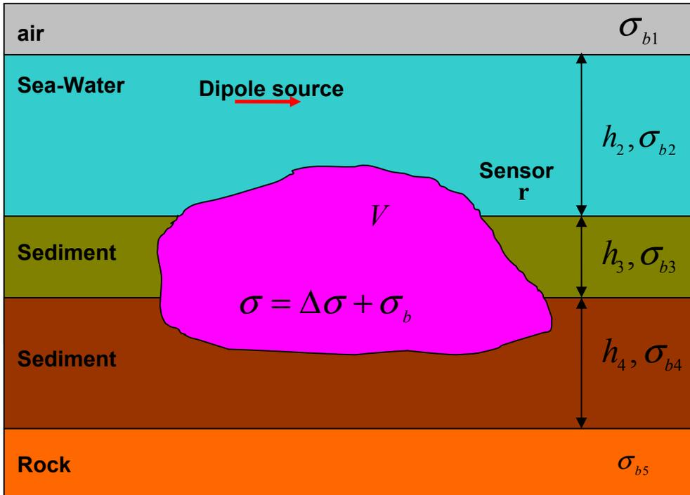
Figure 1. The three-dimensional model of the marine environment consisting of an inhomogeneity with arbitrary conductivity in a stratified background.
