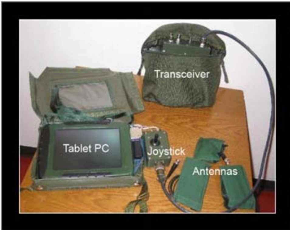
Figure 4: Computer, transceiver, antennas and joystick.
