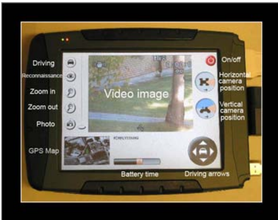
Figure 3: The Field Tablet PC with its functionality.
