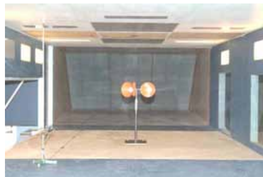
Figure 9 – The largest red rotor in the Gävle WT. Blockage approx. 2.5%
