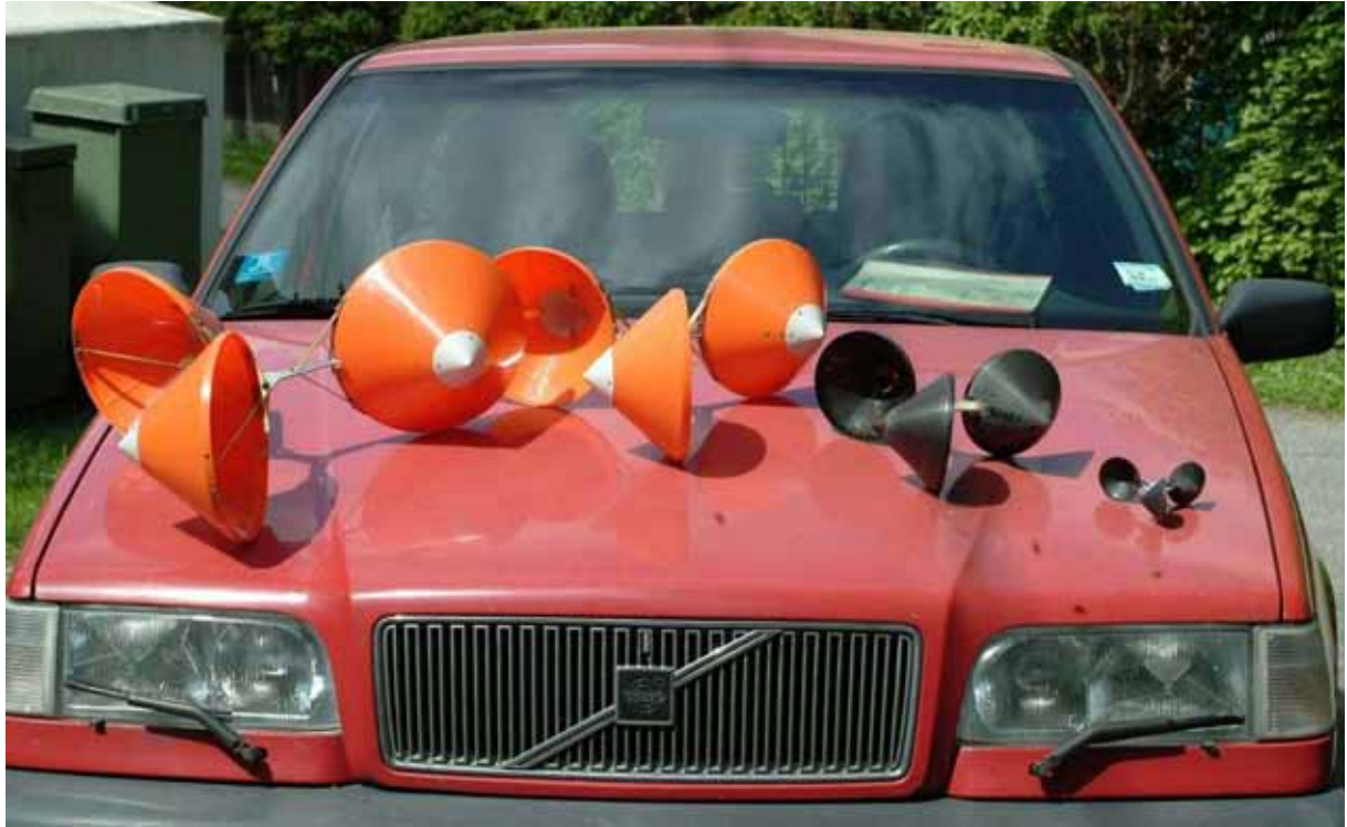
Figure 1 - The cup anemometers lying on the front of a Volvo car provides an impression of the cup sizes. The largest rotor (on the left) could unfortunately not be used because it was too heavy and could jeopardize the anemometer shaft and bearings.
