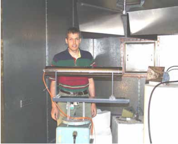
Figure 4.1: A typical Radiated Susceptibility Test (RST). One of the antennas transmits electromagnetic energy into the Reverberation Chamber (RC). The other antenna measures the stress we put onto the Equipment Under Test (EUT). (In this figure the generic missile GENECE is the EUT. The author is to be taken out of the chamber before the test is performed.)
