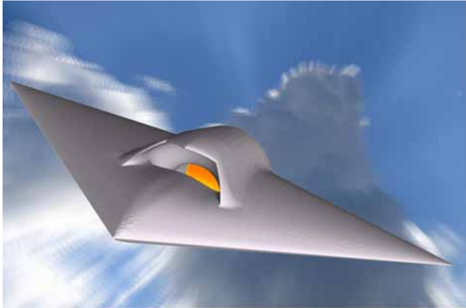
Figure 4.11: EIKON, final design including inlet.
