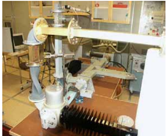
Figure 15. Magnetron, adjustable power splitter, coupler and waveguide switch.
