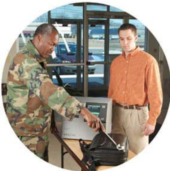
Figure 12 Swiping a bag for particles for detection with Smiths Detection IonScan 400B (Courtesy of Smiths Detection.)
