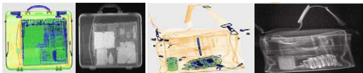
Figure 5 Two ictures on left: The Z Backscatter image of a laptop in a briefcase clearly shows 3 concealed organic -- IEDs hidden in a laptop. The dual-energy transmission image is able to see fine details of the laptop, but it does not detect the organic material hidden in the dense electronics of the laptop. Note: Dual-energy X-rays color organic materials as orange, mixed materials as green, and metallics as blue. Two pictures on right: Gemini's Z Backscatter reveals $4,000 worth of illegal drugs concealed in a PDA and 10 feet of detonator cord wrapped around a laptop power cord - both of which the dual-energy image missed. Courtesy of American Science and Engineering, Inc. ©2006
