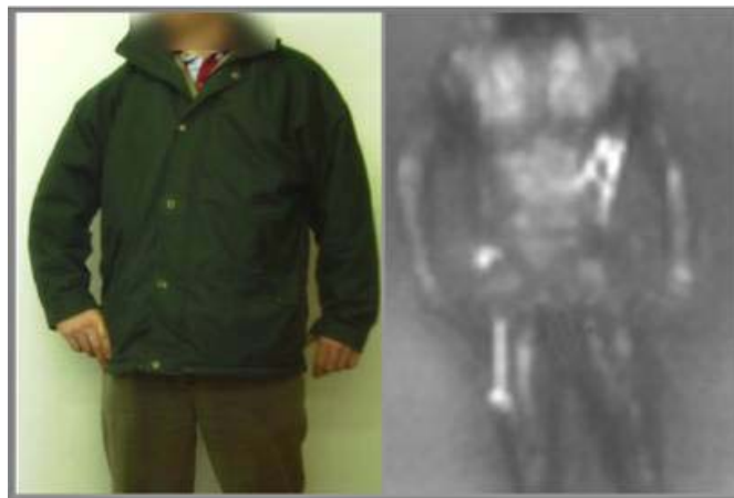
Figure 9 Visualization of threat objects hidden under clothing by means of mm-wave technology. (Courtesy of Smiths Detection).
