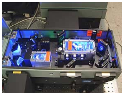
Figure 22 Setup for Cavity Ring Down Spectroscopy (Courtesy of Paul J. Dagdigian and Christopher Ramos, Johns Hopkins University 96 ).
