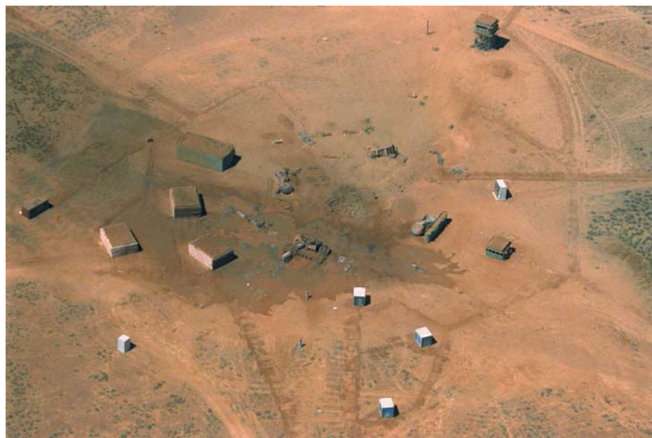
Figure 2 The donor-acceptor set-up of the 5-tonne trial, with the water barrier on the right, next to the donor container.
