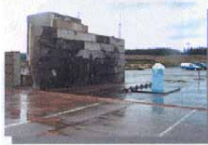
Figure 6 Hydro Suppressor System of Battelle, creating a “water barrier wall”..
