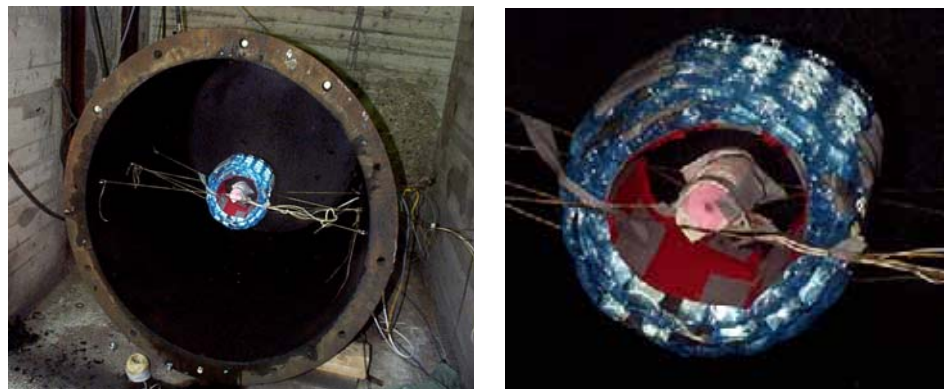
Figure 2. Experimental set-up of charge enclosed by water barrier
