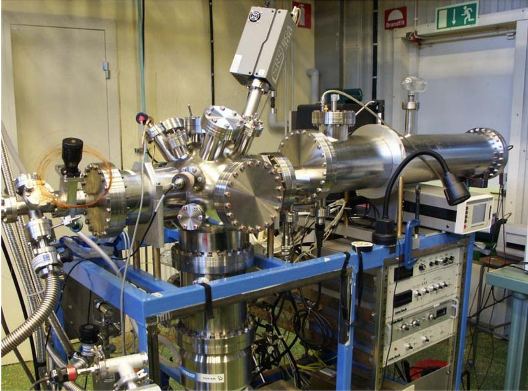
**Figure 3** *The TOF-MS has been equipped with a capillary column feed through. The capillary terminates in the ionization chamber.*
