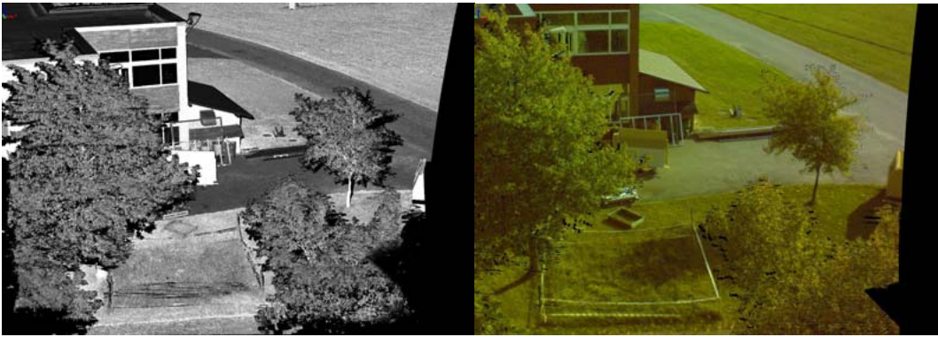
Figure 37. The same point cloud textured with intensity at 1541 nm (left) and RGB (right).
