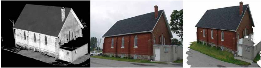
Figure 40. Photo draping of a church. Polygon model to the left and visual photo in the middle are fused together to a photo draped model to the right. (Data and photo from Optech.)
