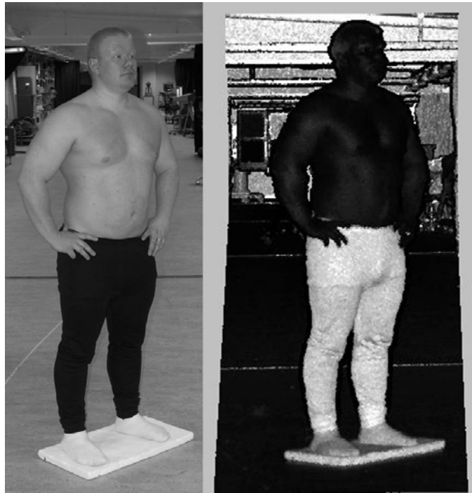
Figure 27. Visual image to the left and to the right an intensity image from ILRIS. Notice the very low reflectance from human skin and the high reflectance from the clothes (from black to white in intensity the reflectance goes from low to high)
