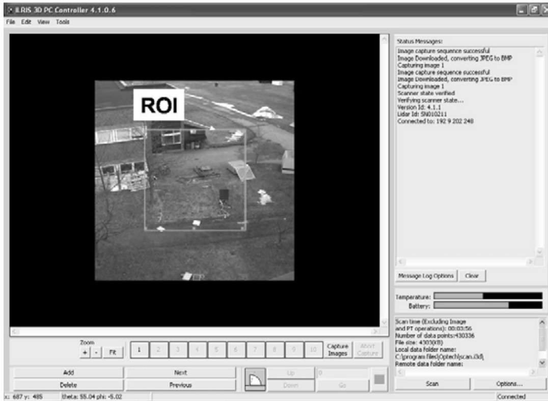
Figure 15. The Controller program interface. The square in the image from the internal video camera shows a ROI set by the operator.
