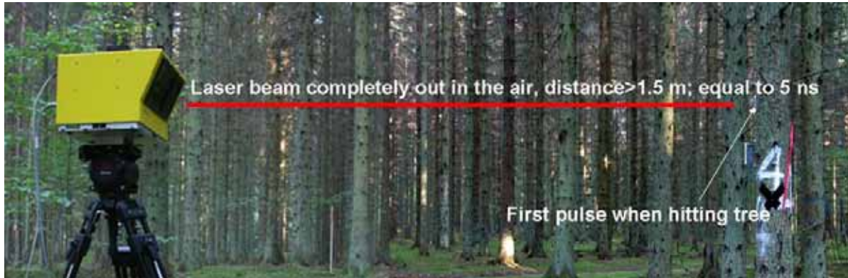
Figure 10. The laser pulse is entirely out in the air before the detection algorithm allows detection.
