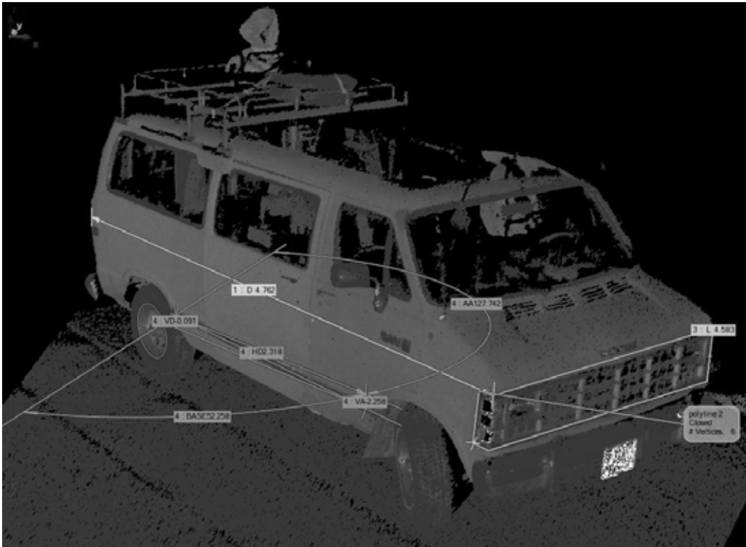
Figure 35. Image shows an example of some measurements made in the Inspect module. Survey measurement shows azimuth, bearing, and vertical angle of vehicles left side compared to scanner position. The lengths of the vehicle, the radius of the rim, the circumference of the grill are some other examples of measurements.
