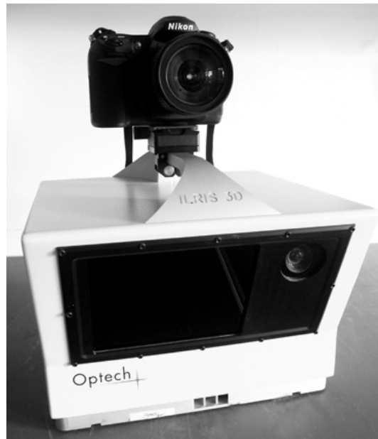
Figure 39. External camera Nikon D200 mounted on ILRIS
