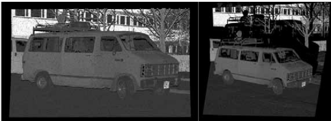
Figure 3. To the left a point cloud viewed in the same direction as the recording was made (the image will look 2-D). To the right the same point cloud rotated from the recording direction.
