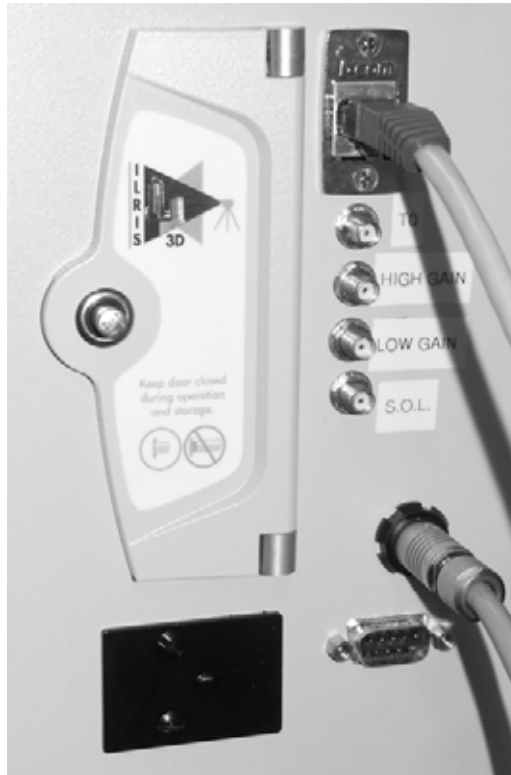
Figure 14. The connectors at the back of ILRIS. To the upper left is a door covering two USB connectors for memory stick, in the lower left is an antenna for WiFi. Upper right is an Ethernet connector. Below that are four SMA Bulk head connectors for analogue outputs and below that there is a power connector and the lower right is a serial connector.
