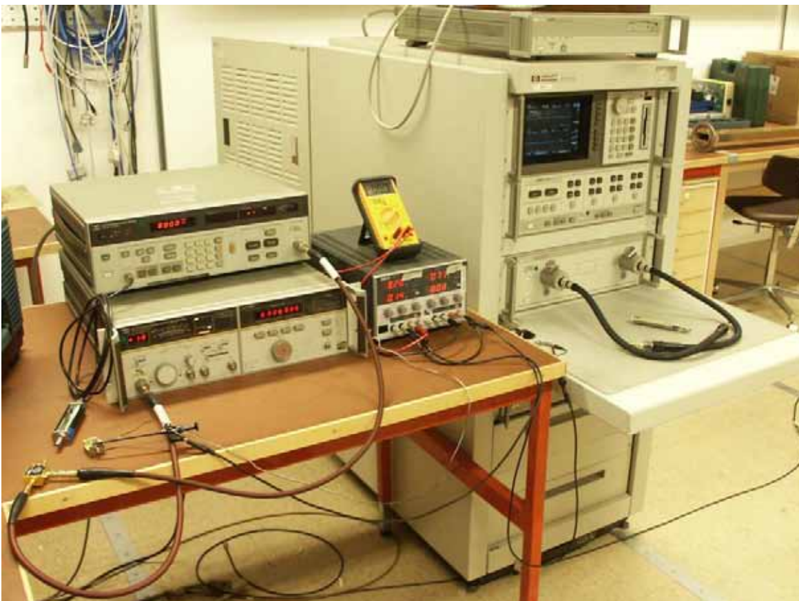
Figure 5.1 Photograph of the measurement setup for noise figure (left) and S-parameters (right).
