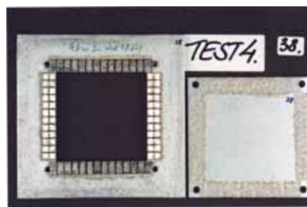
Figure 21: Test object with clear chromated aluminum/tin plated contact fingers after exposure to accelerated corrosion test.
