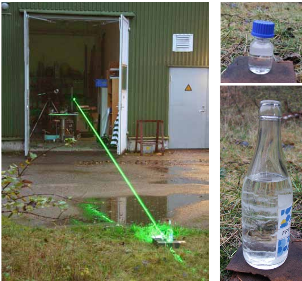
Figure 15: Outdoors experiment on nitromethane in a standard 33 cl soft drink bottle. The telescope can be seen to the left of the mirror directing the laser beam. The bottle used for nitromethane and the smaller bottle of Pyran used for nitrobenzene and isopropyl nitrate is seen to the right.
