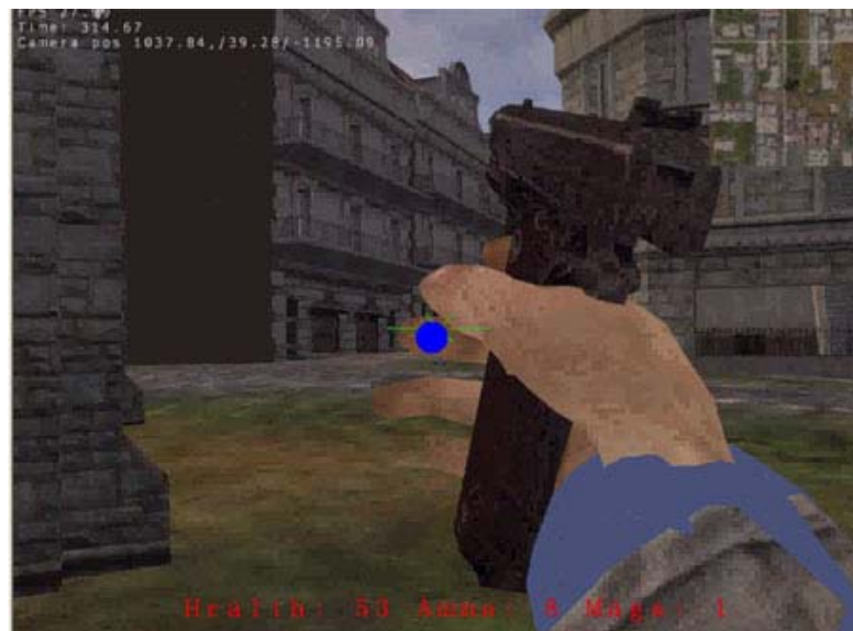
Figure 25. Here the ray-trace goes through the finger graphic and picks the house object in the prolonged direction behind it [row 14,144 / frame 3,129].
