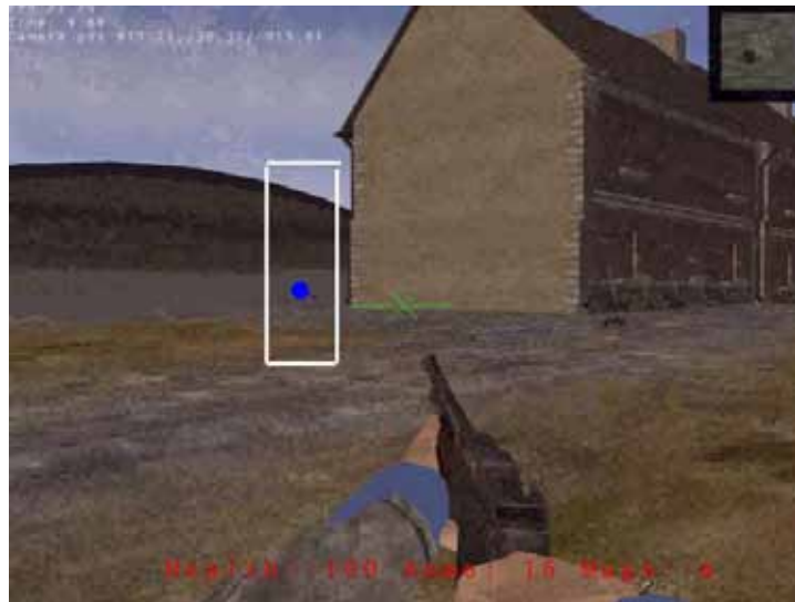
Figure 34. In this case the wall/fence does not have any collision detection and therefore, since the object under the gaze point is detected by the engine using a collision volume/surface, the hangar is logged instead.
