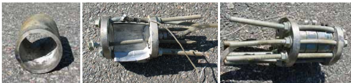
Figure 9. Test setup after cook-off: cylinder (left), setup showing the opened side of the heating band (middle) and setup showing the back side of the heating band (right).
