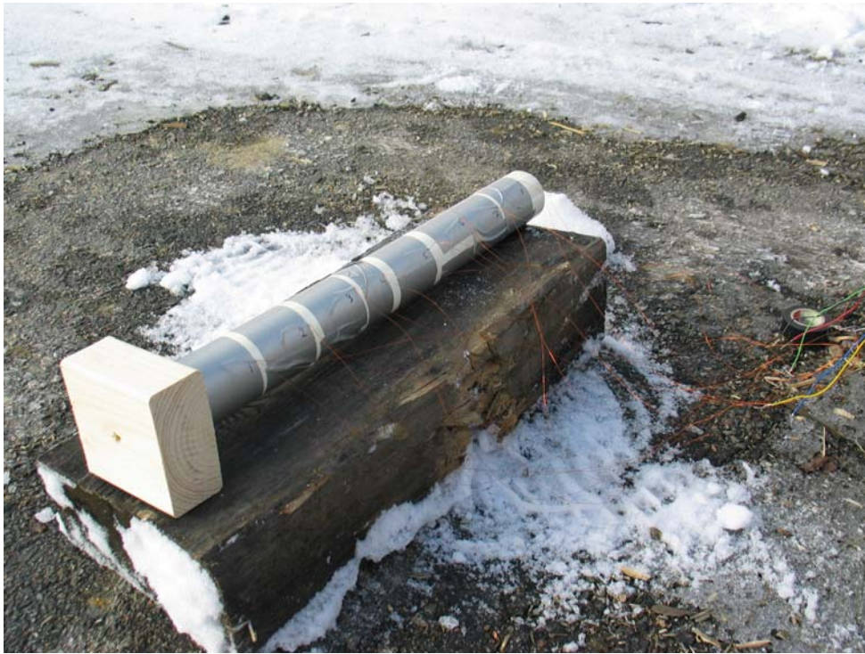
Figure 4. Setup for measuring the detonation velocity.
