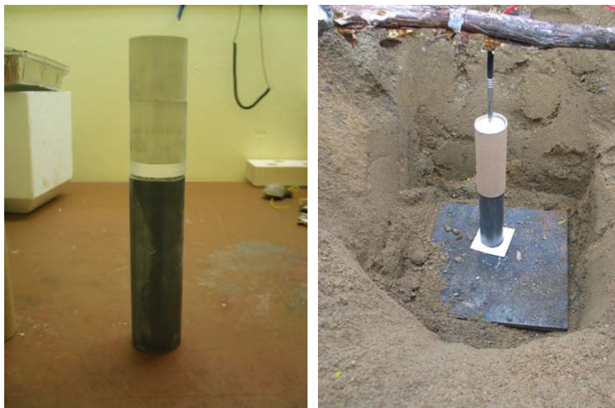
Figure 9. Booster charge (top, left), cards (middle, left) and FOX-12 donor charge in a steel cylinder (bottom, left). Large scale gap test setup before test (right).
