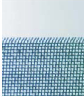
Figure 3.9. Stainless steel mesh electrode used by Takashi Abe et al. in order to enhance the electric field close to the electrode surface and obtain a higher density of ions. This method proved to be about 50 % more efficient than using a simple metal foil of the same thickness. The thickness of the mesh is 25 \mu\text{m} .
