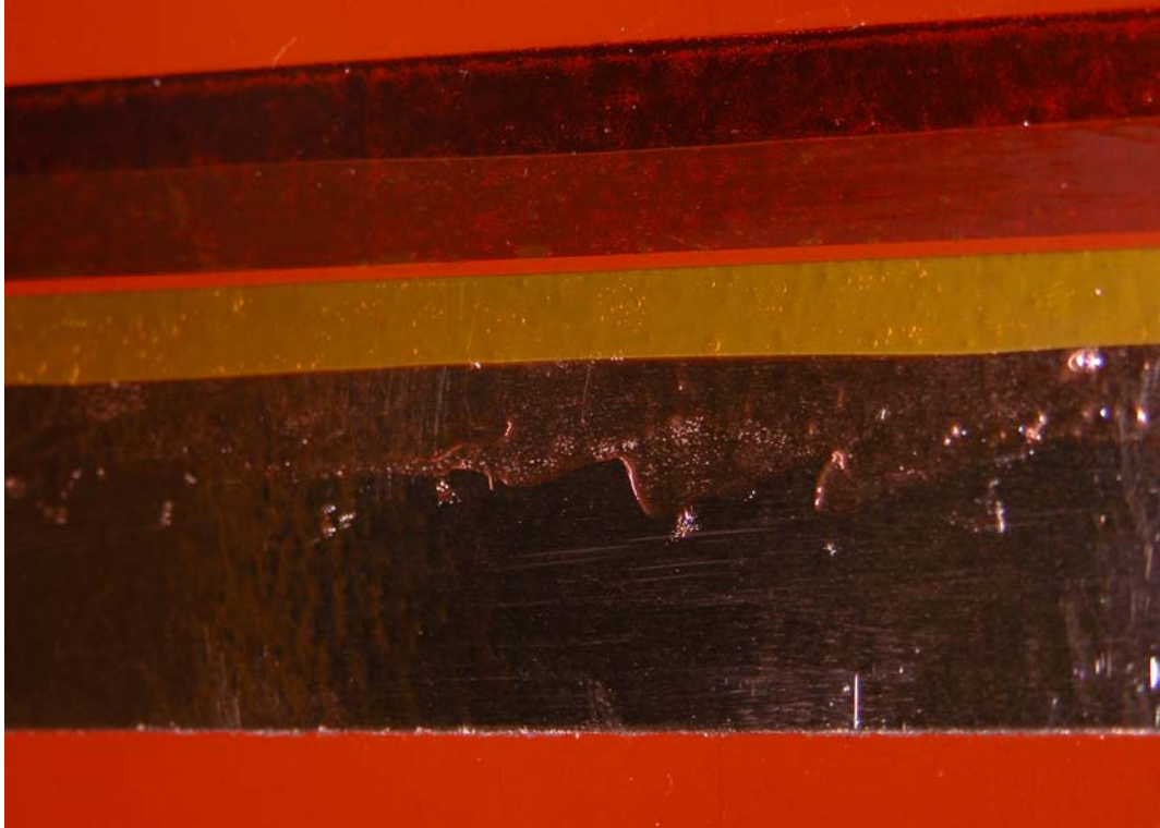
Figure 3.2. Close up on backside of plasma actuator. The edge of the bottom electrode is covered with Epoxi glue and a piece of CR200 Kapton covers the edge to prevent any plasma formation. Plasma formation on the 'backside' of the actuator will cause erosion of the surface beneath the actuator, it will also lower the efficiency of the actuator because of the extra energy spent on ionizing the air trapped between the actuator and the surface below.
