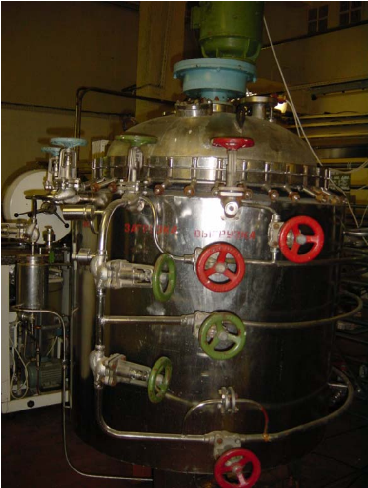
Fermentation vessel at former BW plant (Photo K. S. Westerdahl FOI)
