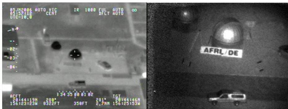
Simultaneous nighttime co-boresighted FLIR image (Left) and Laser SWIR photo (Right). Note reading signs, bar targets, ladder, Positive ID of Nissan with Campershell from laser
