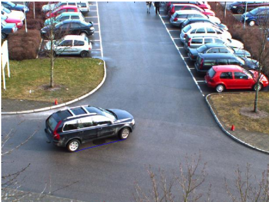
Figure 6.6: The wheelbase of a Volvo XC90 is marked with a thin blue line.
