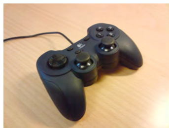
Figure 4.3: A gamepad with two joysticks. Control devices of this type are used for computer games and in recent times also for teleoperation control of robots such as the Irobot Packbot in Figure 4.2. This gamepad was furthermore used in the evaluations in Section 4.3.
