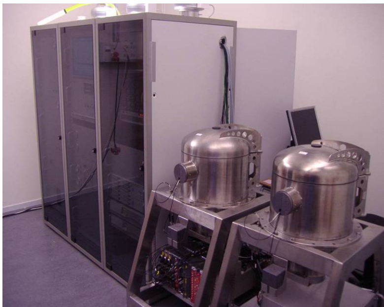
Fig. 5: The automatic radioxenon system SAUNA II belonging to the International Monitoring System and operated by FOI.
