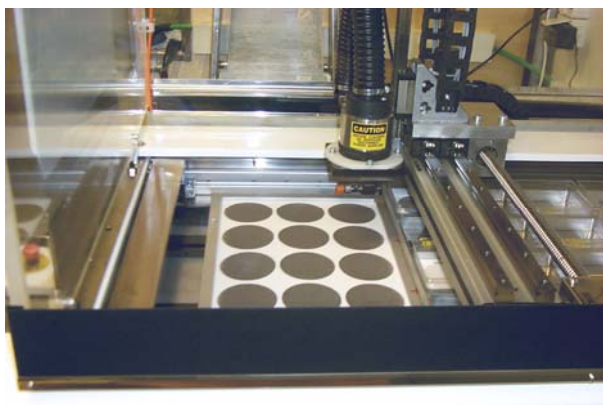
Fig. 4: The robot arm cutting and moving the filter pieces in the CINDERELLA system used in the CTBTO station SEP63.
