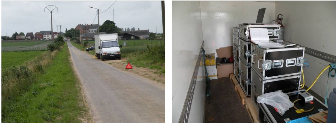
Fig. 10: The lorry used to carry the mobile radiocesium sampling equipment parked during sampling (left). The right picture shows the interior of the lorry with the mobile sampling equipment.
