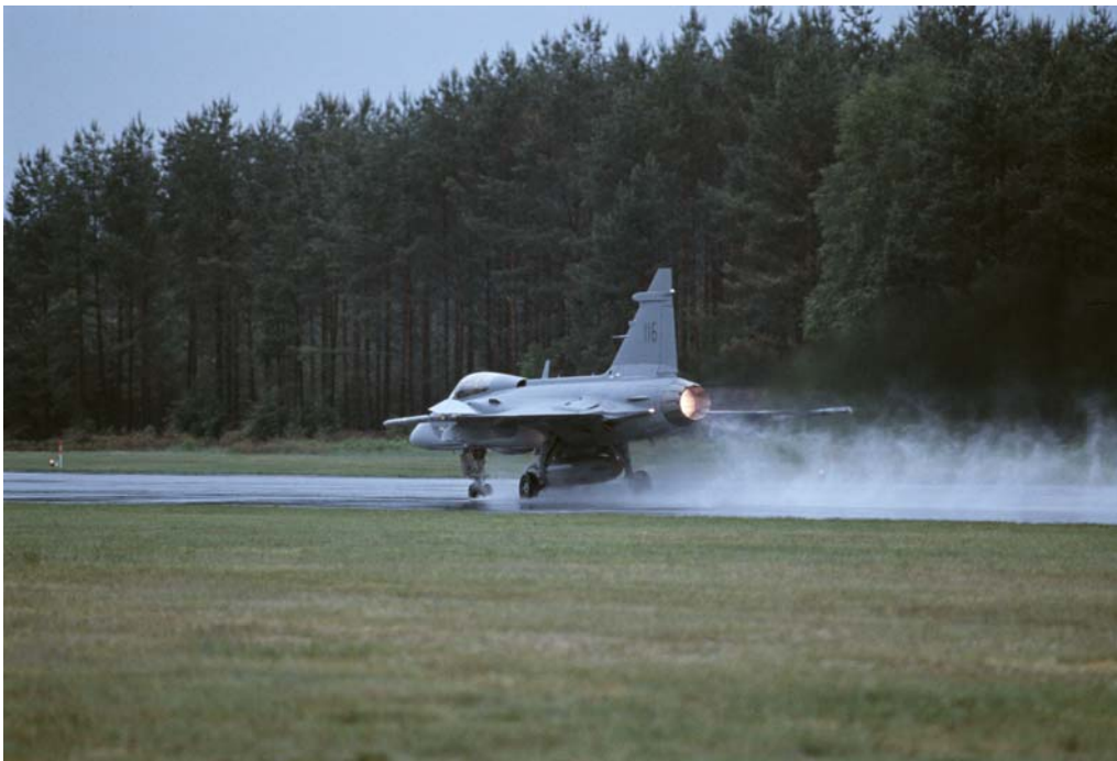
Figure 1. Gripen fighter during start. The upper limit of the area affected by the turbulence from the engine exhaust can be seen by the distortion of the trees in the background. Water droplets from the wet runway disturb the lower part of the image. (Photo: Peter Liander - Försvarets Bildbyrå)
